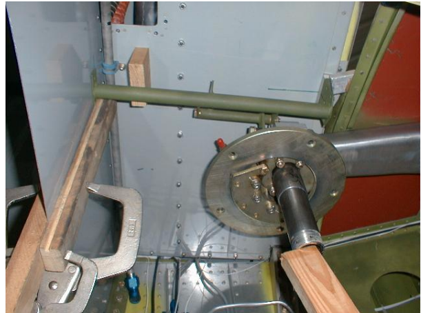
Figure 3.17. The uplock carry structure held in place with clamps.
