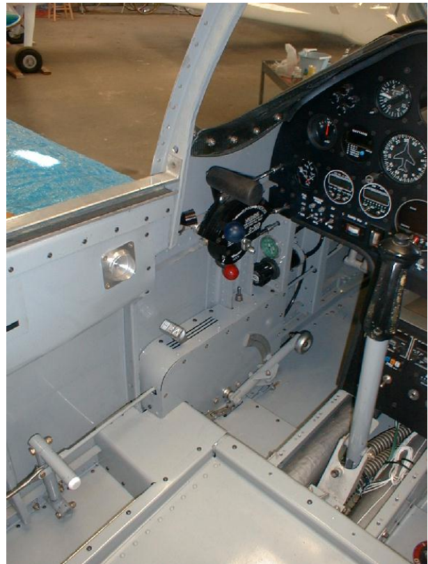
Figure 3.14. In this example the controls for heat, defrost and air are put in the console.
