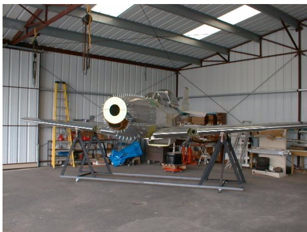
Figure 3.3. The airframe mounted on the wingstands. If you join the stands together with angle iron and add heavy duty casters, you can roll the wings under the fuselage.
