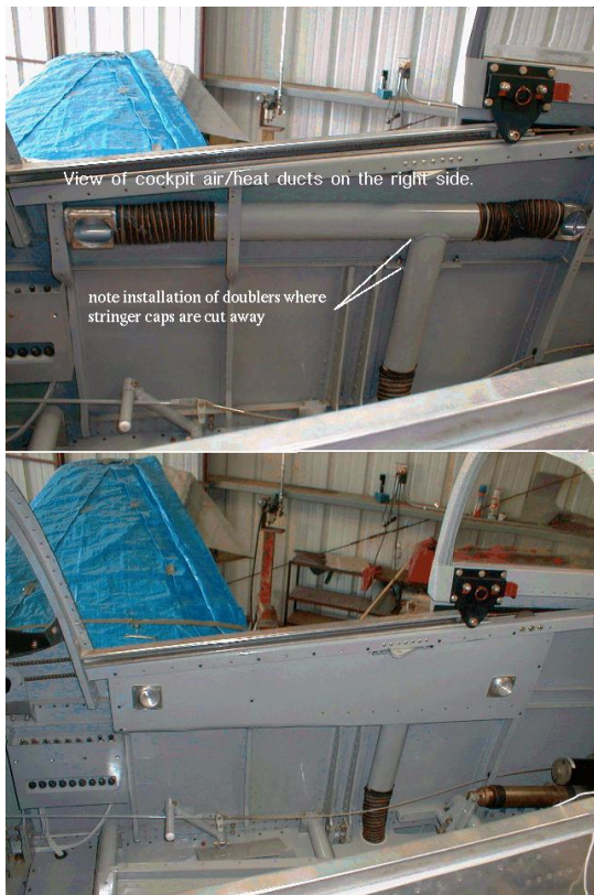
Figure 3.12. An example of a duct constructed from tubing.
