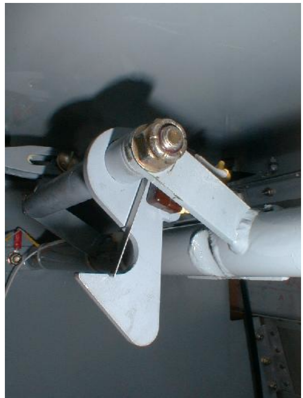
Figure 3.20. The main gear uplock microswitches mount on the unlock hooks.
