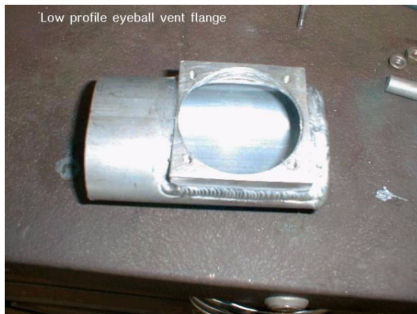
Figure 3.13. Low profile flanges to mount the eyeball vents.
