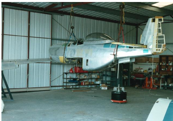
Figure 3.4. The fuselage suspended from chain hoists.
