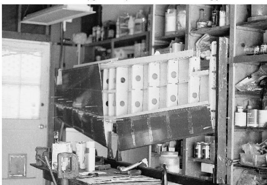
Figure 2.40. The horizontal stabilizer in the assembly jig.
