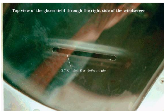
Figure 2.34. View of the defroster slot in the right glareshield looking down through the side windscreen. The defrost air is directed towards the side windscreen sections only.
