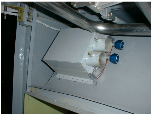
Figure 2.24. Heater plenum installed on the duct. This example uses a GM aluminum heater core, and controls the coolant flow with a butterfly valve. The ducts route air (heated or unheated) separately to the cabin and windshield defroster. If you want to use this arrangement, keep in mind that you may eventually want to put the battery in this same general area. This might make for a tight fit.
