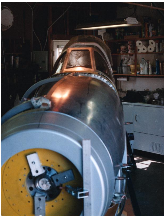
Figure 2.51. The aft part of the spinner mounted on the prop hub with some crude clamps. The forward cowl bulkhead gets clamped to the spinner backing plate and locates the front of the cowl.
