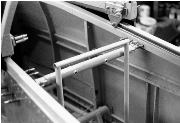
Figure 2.38. The cross-strut supports the back of the front seat and anchors the pilot's shoulder harness. Use a pin in one side so it can be pivoted out of the way for back seat entry and egress.
