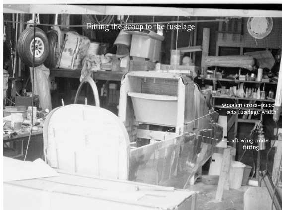
Figure 2.19. Fit the scoop with the fuselage inverted and with internal braces installed as necessary to control the fuselage width.
