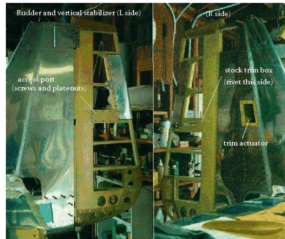
Figure 2.44. Here the actuator is installed in the vertical stabilizer and a push-pull cable is used to move the trim tab.
