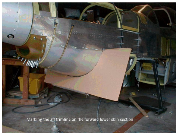
Figure 2.56. Preparing to trim the aft end of the lower forward cowl skin. Just mark the plane of the cardboard and trim along the line.
