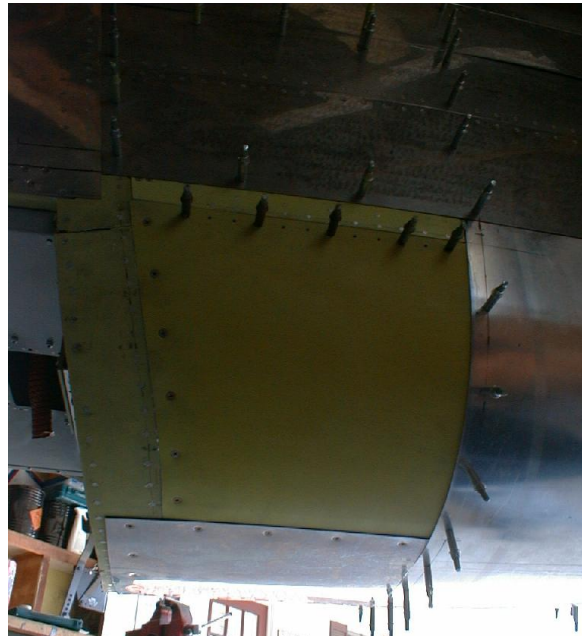
Figure 2.57. View of the lower aft cowl section from the lower right. This skin section is cut into three pieces. The outboard pieces underlap the middle skin section. A minimum of 1.5" should be allowed at the lap joint to install Dzus fasteners.
