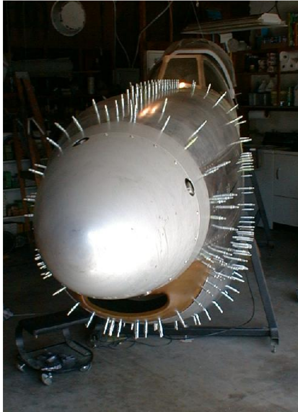
Figure 2.58. Here the cowling is nearly ready for installation of Dzus fasteners. You may need to do a little forming where the lower cowl mates with the chinscoop. This shows the joint before "adjustment".
