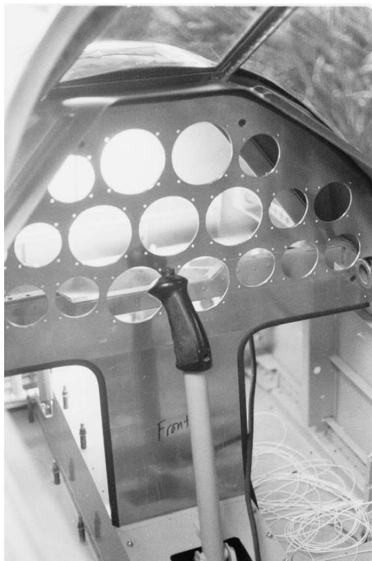
Figure 2.32. This instrument panel is fabricated from 0.125" 6061-T6.
