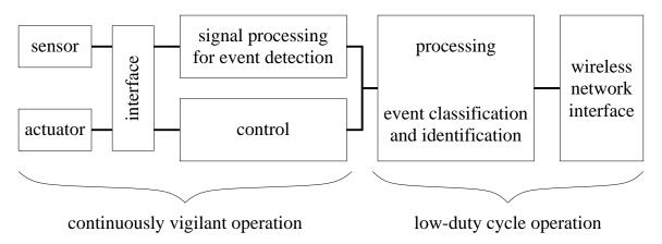
Figure 1. The architecture of a sensor node
