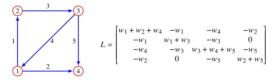
this is the conductance matrix of a resistive circuit ( $w_k$  is conductance in branch k)
