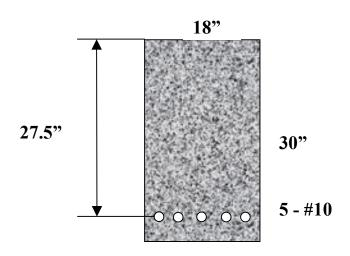
2.2 For the following sections, compute  $\phi M_n$ . Also compute the depth of the neutral axis, the curvature, and the strain in the reinforcement (for a maximum compression strain of 0.003). Use 1.5" cover and assume #3 stirrups for all cases. For case (b), the beam has a 2"x8" opening.
