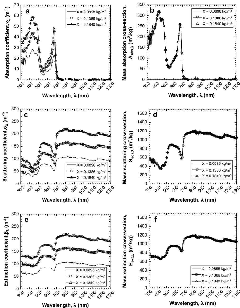
Fig. 6 – The (a) absorption  $\kappa_\lambda$ , (c) scattering  $\sigma_\lambda$ , and (d) extinction  $\beta_\lambda$  coefficients and the corresponding (b) mass absorption  $A_{\text{abs},\lambda}$ , (d) mass scattering  $S_{\text{sca},\lambda}$ , and (f) mass extinction  $E_{\text{ext},\lambda}$  cross-sections of *C. reinhardtii* CC125 over the spectral range from 300 to 1300 nm at three different microorganism concentrations.
