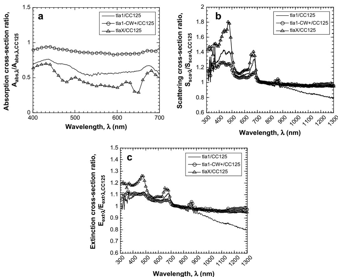
Fig. 10 – The ratio of the (a) mass absorption  $A_{\text{abs},\lambda}$  (b) mass scattering  $S_{\text{sca},\lambda}$  (c) mass extinction cross-sections  $E_{\text{ext},\lambda}$  of *tla1*, *tla1-CW<sup>+</sup>* and *tlaX* with respect to those of *C. reinhardtii* CC125.
