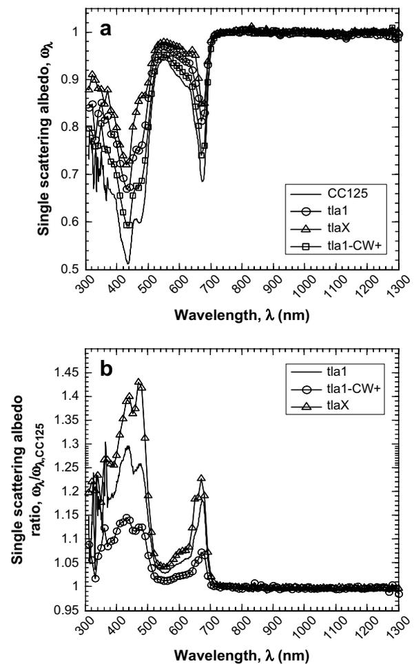
Fig. 11 – (a) The single scattering albedo  $\omega_\lambda$  for all strains and (b) the ratio of the single scattering albedo of *tla1*, *tlaX* and *tla1-CW<sup>+</sup>* with respect to that of *C. reinhardtii* CC125 over the spectral range from 300 to 1300 nm.
