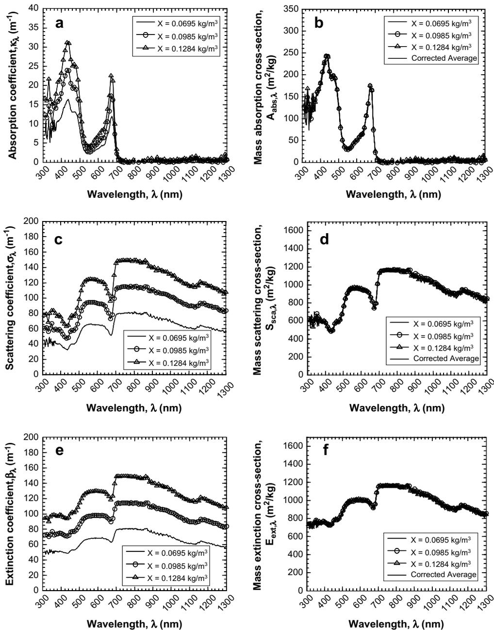
Fig. 7 – The (a) absorption  $\kappa_\lambda$ , (c) scattering  $\sigma_\lambda$ , and (d) extinction  $\beta_\lambda$  coefficients and the corresponding (b) mass absorption  $A_{\text{abs},\lambda}$ , (d) mass scattering  $S_{\text{sca},\lambda}$  and (f) mass extinction  $E_{\text{ext},\lambda}$  cross-sections of *C. reinhardtii tla1* over the spectral range from 300 to 1300 nm at three different microorganism concentrations.
