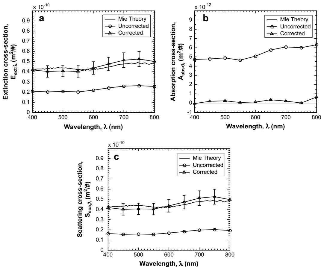
Fig. 5 – Comparison of the experimentally measured uncorrected and corrected (a) extinction, (b) absorption, and (c) scattering cross-sections of  $5 \mu\text{m}$  diameter polystyrene microspheres with those predicted by the Mie theory.
