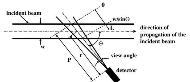
**Fig. 4 – Coordinate system used in recovering the scattering phase function from the measured intensity distribution [26].**
