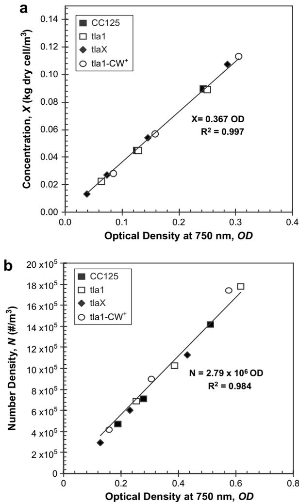
**Fig. 3 – Calibration curves of (a) dry cell weight and (b) number density versus optical density (OD) at 750 nm for all strains.**
