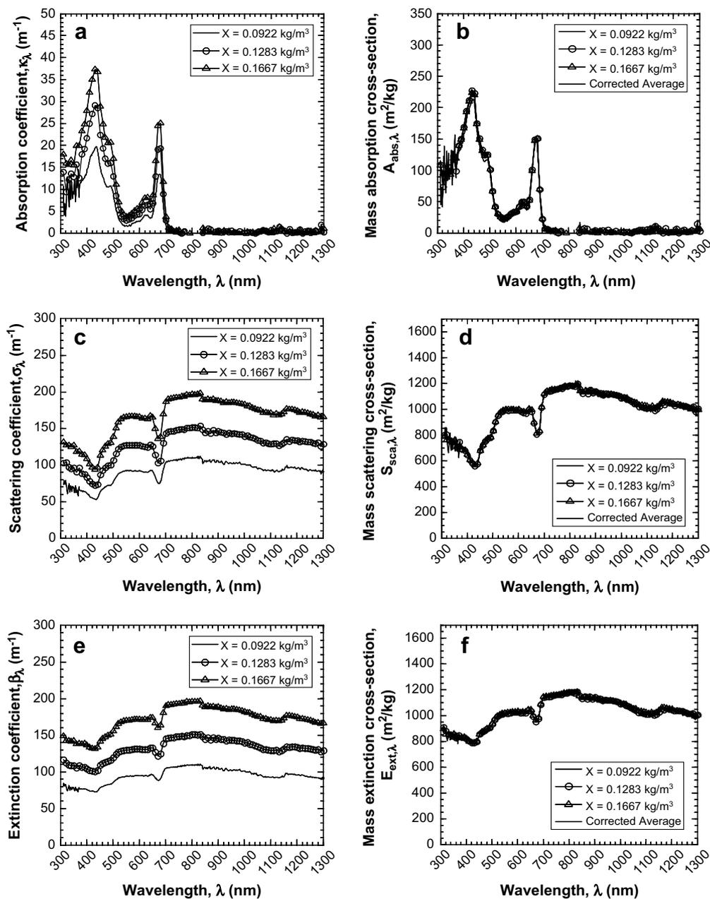
Fig. 8 – The (a) absorption  $\kappa_\lambda$ , (c) scattering  $\sigma_\lambda$ , and (d) extinction  $\beta_\lambda$  coefficients and the corresponding (b) mass absorption  $A_{\text{abs},\lambda}$ , (d) mass scattering  $S_{\text{sca},\lambda}$  and (f) mass extinction  $E_{\text{ext},\lambda}$  cross-sections of *C. reinhardtii* tlaX over the spectral range from 300 to 1300 nm at three different microorganism concentrations.
