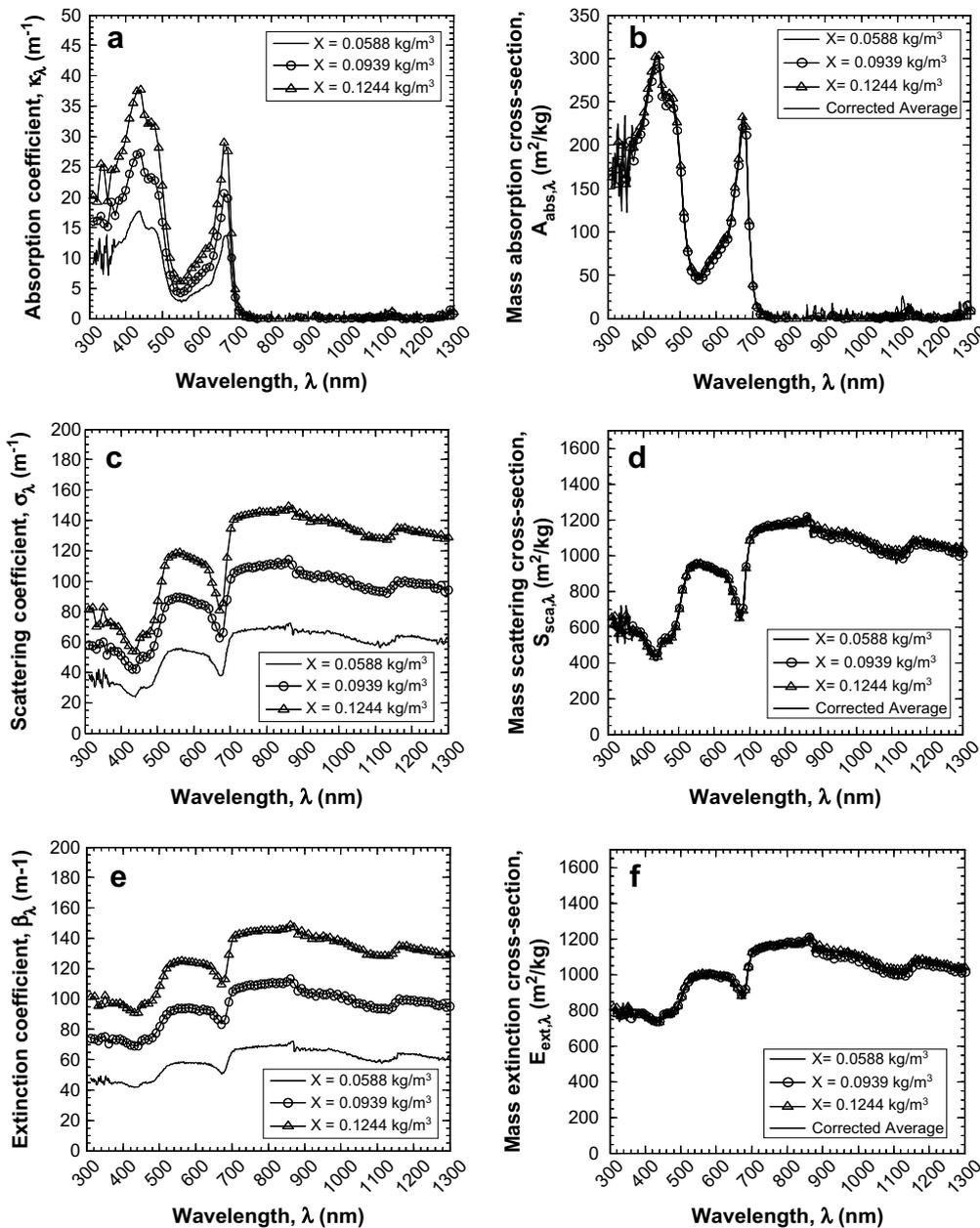
Fig. 9 – The (a) absorption  $\kappa_\lambda$ , (c) scattering  $\sigma_\lambda$ , and (d) extinction  $\beta_\lambda$  coefficients and the corresponding (b) mass absorption  $A_{\text{abs},\lambda}$ , (d) mass scattering  $S_{\text{sca},\lambda}$  and (f) mass extinction  $E_{\text{ext},\lambda}$  cross-sections of *C. reinhardtii* tla1-CW<sup>+</sup> over the spectral range from 300 to 1300 nm at three different microorganism concentrations.
