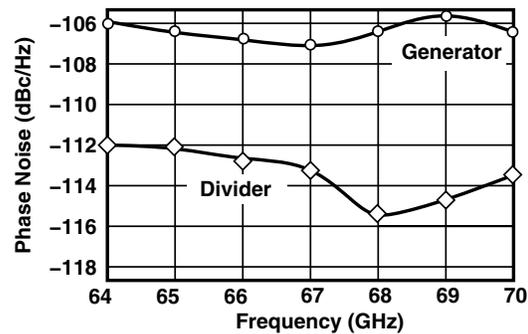
Fig. 10. Measured phase noise of divider.
