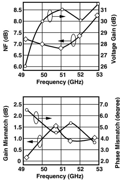
Fig. 5. Measured receiver performance.
