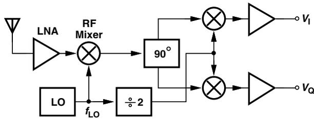
Fig. 1. Receiver architecture.
