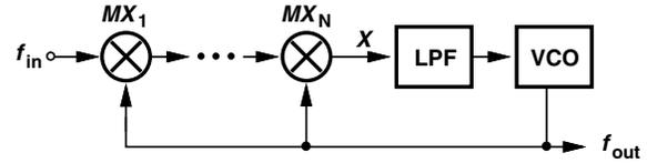
Fig. 6. Heterodyne phase-locked loop.
