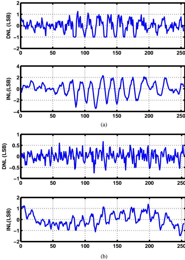
Fig. 8. Measured DNL and INL at a clock rate of 4 GS/s, (a) before, and (b) after per-channel calibration.
