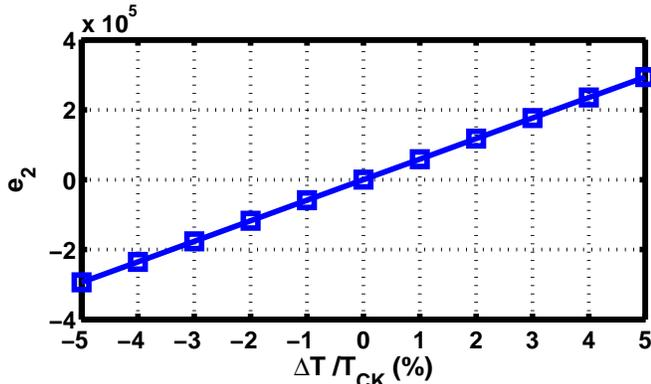
Fig. 3. Simulated error as a function of timing mismatch (arbitrary vertical scale).
