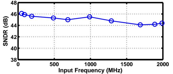
Fig. 12. Measured SNDR as a function of  $f_{in}$  at 4 GS/s.
