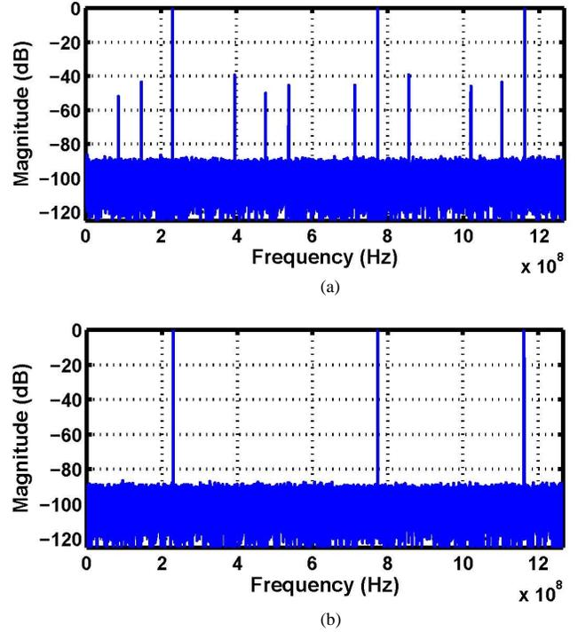
Fig. 4. Simulated ADC output spectrum (a) before, and (b) after calibration for a multi-tone input.
