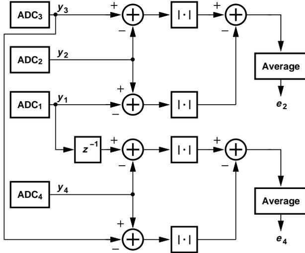
Fig. 2. Timing mismatch detection in a 4-channel ADC system.
