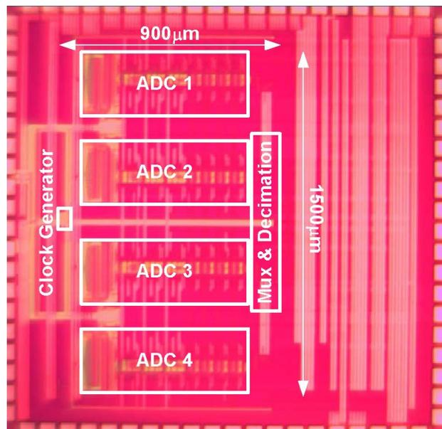
Fig. 7. Prototype ADC micrograph.
