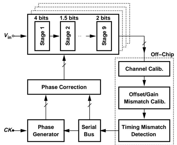
Fig. 5. ADC architecture.
