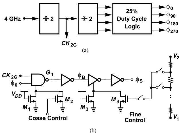
Fig. 6. (a) Phase generation, and (b) phase adjustment circuits.
