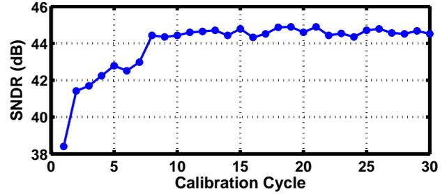
Fig. 10. Measured SNDR during convergence of timing calibration.
