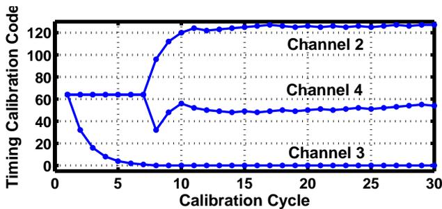
Fig. 9. Measured timing calibration code convergence.
