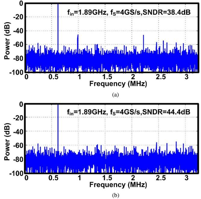
Fig. 11. Measured output spectrum (a) before, and (b) after timing mismatch calibration (decimated by a factor of 625).
