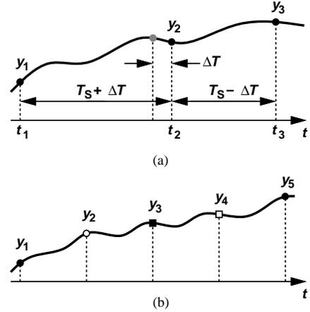
Fig. 1. Waveforms showing effect of timing error in a (a) two-channel or (b) four-channel interleaved ADC system.
