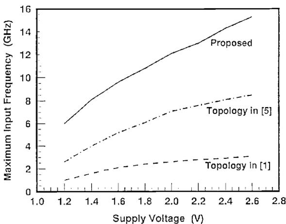
Figure 3: Simulated speed of divider and topologies in [1] and [5].
