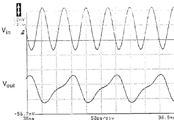
Figure 5: Measured input/output waveforms at 13.4GHz (input amplitude not to scale).
