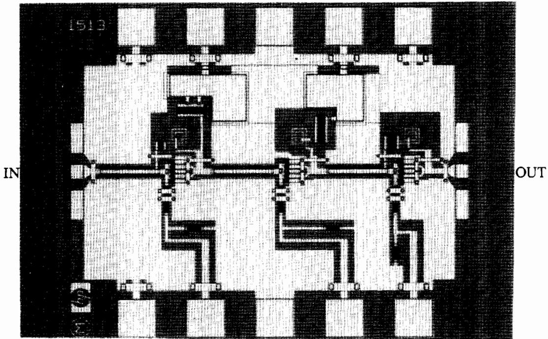
Figure 2: Micrograph of three-stage amplifier.
