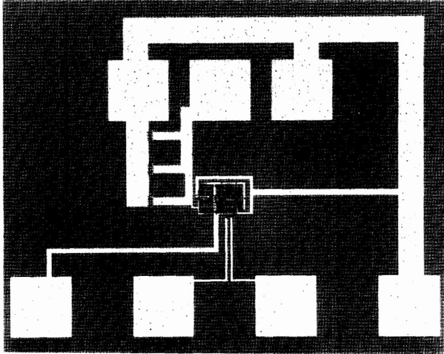
Figure 4: Divider chip micrograph.
