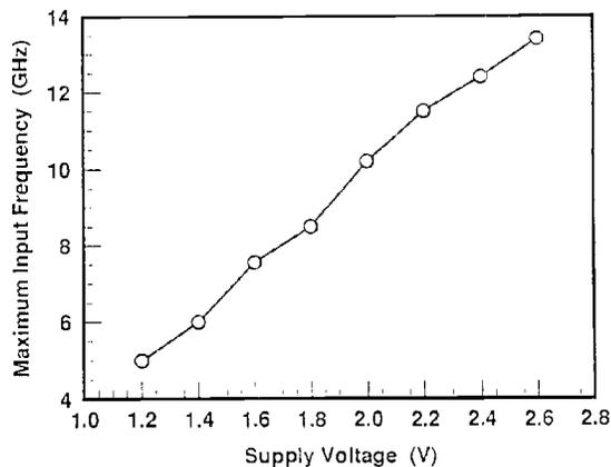
Figure 6: Measured speed vs supply voltage.
