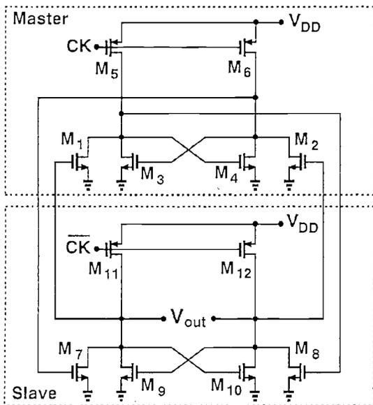
Figure 2: Divider circuit.
