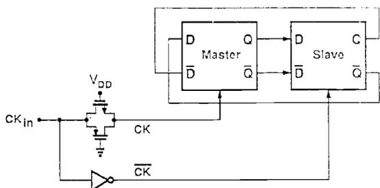
Figure 1: Divider block diagram.
