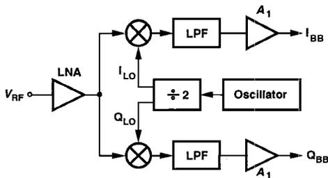
Fig. 1. Receiver architecture.
