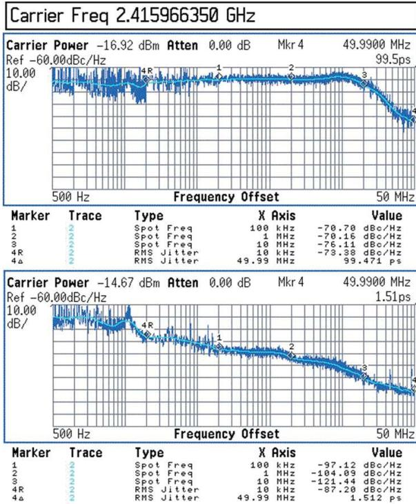
Fig. 21. Measured phase noise in fractional- $N$  mode.
