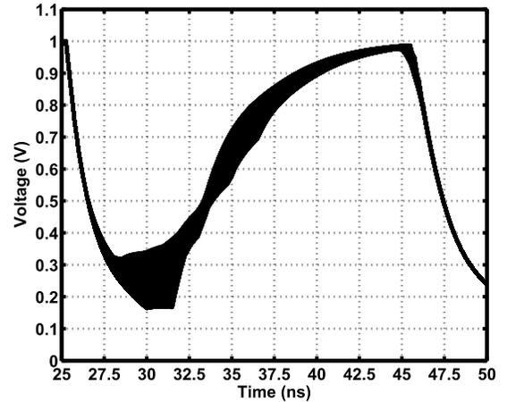
Fig. 5. Eye diagram of filtered output.
