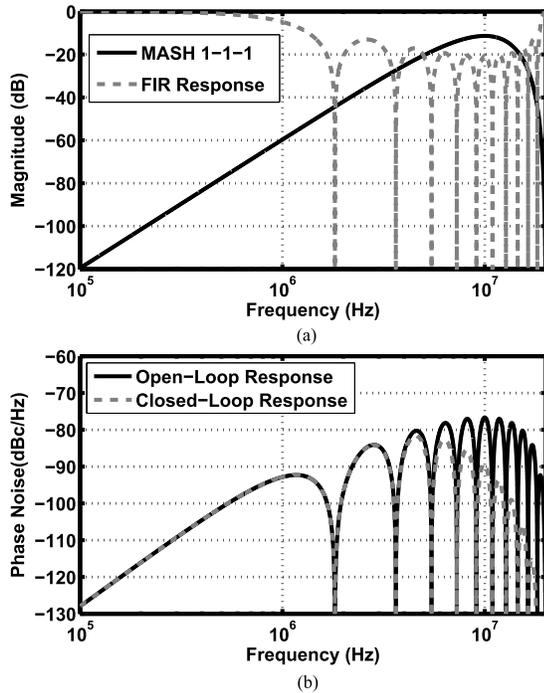
Fig. 6. (a) Output spectrum of MASH 1-1-1 modulator and example of magnitude response for an 11-tap FIR filter. (b) Resulting phase noise plots for open-loop and closed-loop synthesizers.
