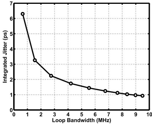
Fig. 17. Simulated integrated jitter versus loop BW.
