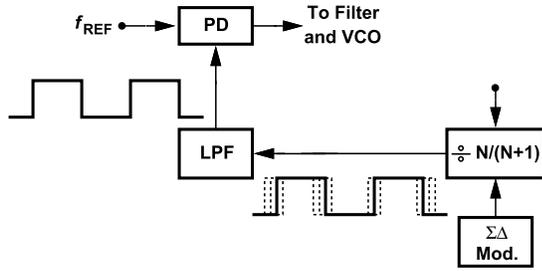
Fig. 2. Suppression of  $\Sigma\Delta$  quantization noise by an LPF.
