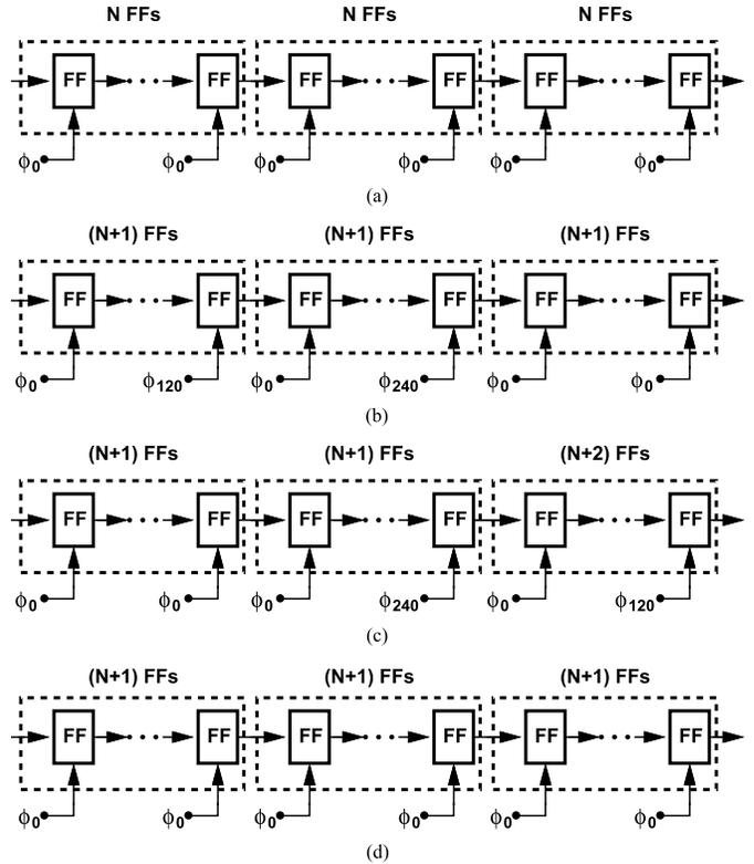
Fig. 15. Delay arrangement when (a)  $\alpha < 1/6$ , (b)  $1/6 \leq \alpha < 1/2$ , (c)  $1/2 \leq \alpha < 5/6$ , and (d)  $5/6 \leq \alpha < 1$ .
