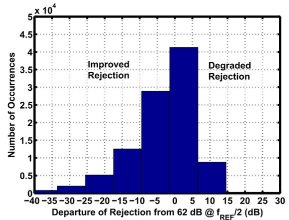
Fig. 8. Monte-Carlo results showing departure of rejection from 62 dB at  $f_{\text{REF}}/2$ .
