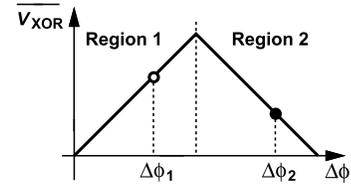
Fig. 14. Nonmonotonic XOR PD characteristic.
