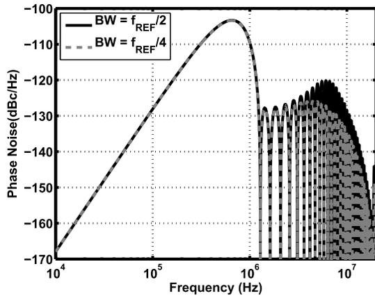
Fig. 10. Synthesizer  $\Sigma\Delta$ -induced phase noise for different loop BWs.
