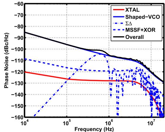
Fig. 16. Overall simulated PLL phase noise and main contributors, all referred to output.
