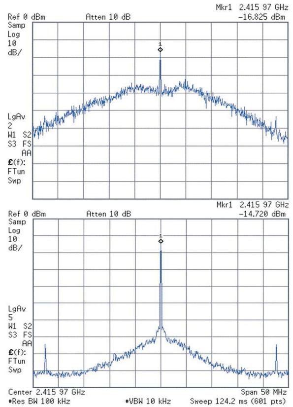
Fig. 19. Measured spectra in fractional-*N* mode with 2-tap FIR (top) and 35-tap FIR (bottom). (Horizontal scale: 5 MHz/div., vertical scale: 10 dB/div.)
