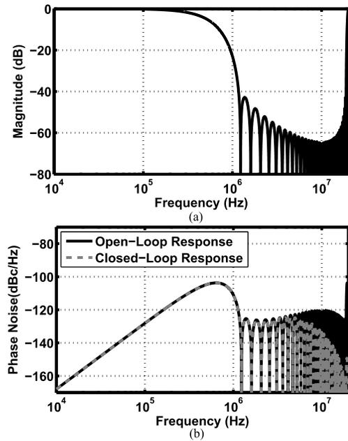
Fig. 7. (a) 35-tap Kaiser-Bessel FIR response. (b) Synthesizer output phase noise due to  $\Sigma\Delta$  contribution.
