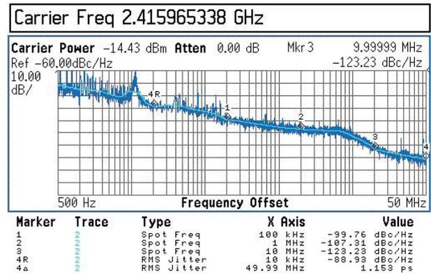
Fig. 20. Measured phase noise in integer-*N* mode.
