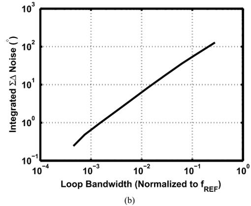
Fig. 1. (a) Synthesizer with MSSF. (b) Integrated noise of a third-order  $\Sigma\Delta$  modulator at PLL output versus loop BW.
