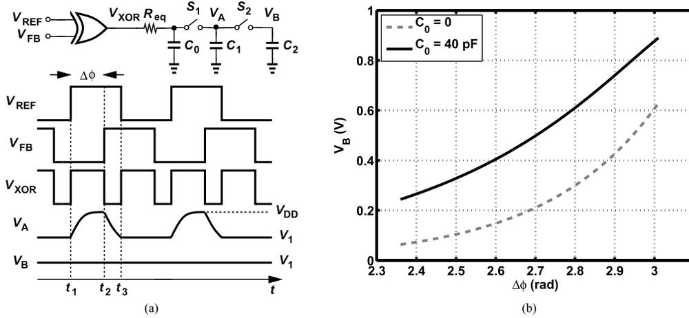
Fig. 12. (a) XOR PD driving MSSF. (b) Control voltage versus static phase error.
