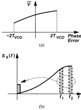
Fig. 24. (a) Nonlinear characteristic of PD. (b) Illustration of noise folding.
