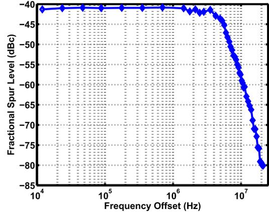
Fig. 22. Measured fractional spur level versus frequency offset.
