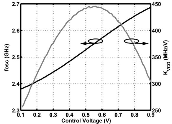
Fig. 11. Simulated VCO frequency and tuning gain versus control voltage.
