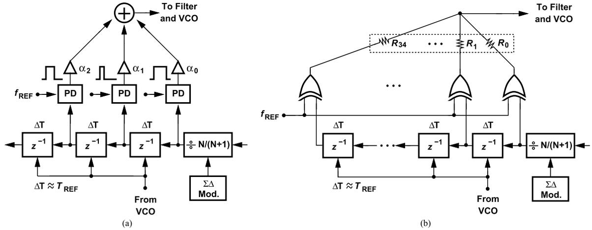
Fig. 4. FIR filter (a) with phase detection, multiplication, and summation and (b) implementation. ( $z^{-1}$  consists of approximately  $N$  flip-flops).
