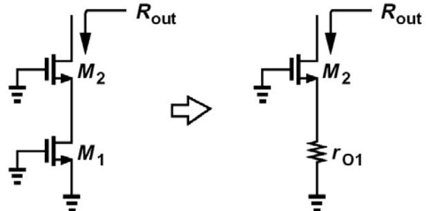
**Cascode Stage with Current Source Load**
