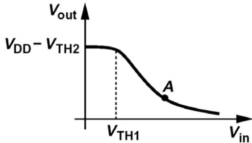
**Example: Common Source with PMOS Diode Load**
