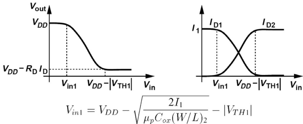
$$V_{in1} = V_{DD} - \sqrt{\frac{2I_1}{\mu_p C_{ox} (W/L)_2}} - |V_{TH1}|$$
