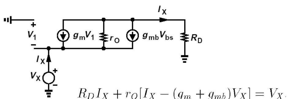
$$R_D I_X + r_O [I_X - (g_m + g_{mb})V_X] = V_X$$
