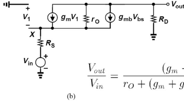
$$\frac{V_{out}}{V_{in}} = \frac{(g_m + g_{mb})r_O + 1}{r_O + (g_m + g_{mb})r_O R_S + R_S + R_D} R_D$$
