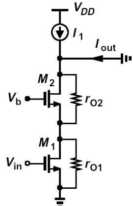
$$I_{out} = g_{m1} V_{in} \frac{r_{O1}}{r_{O1} + \frac{1}{g_{m2} + g_{mb2}} || r_{O2}}$$
