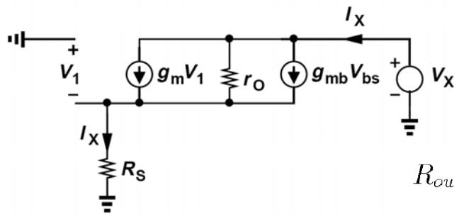
$$\begin{aligned} R_{out} &= [1 + (g_m + g_{mb})R_s]r_O + R_s \\ &= [1 + (g_m + g_{mb})r_O]R_s + r_O. \end{aligned}$$
