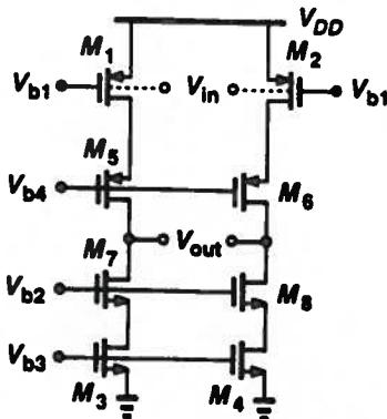
(a) Fully symmetric  $\Rightarrow$  use half circuit.
