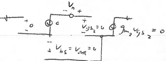
Noise of  $M_2$  doesn't appear at the output (suppressed by the  $\infty$  voltage gain from  $V_{out}$  to the drain voltage of  $M_1$ )
