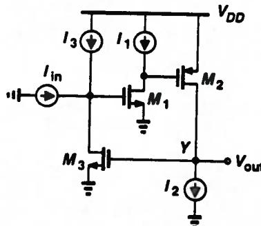
(a) V-C Feedback: use Y model:  $Y_{21} = g_{m3} = \beta$ ,  $Y_{22} = k_{T3}$ ,  $Y_{11} = 0$
