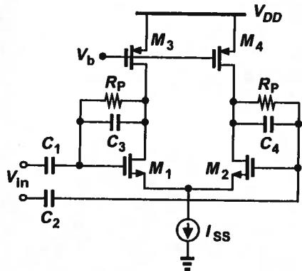
(a) Each output node can swing by  $\pm V_{TH}$  around the CM level  $\Rightarrow$  total diff. swing =  $\pm 2V_{TH}$ .
