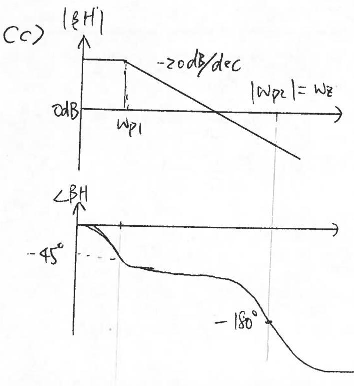
The 0dB point should be between  $\omega_{p1}$  and  $\omega_{p2}$ , so that we have a reasonable phase margin. (d) depends on this notion.
