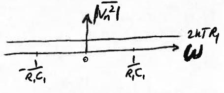
$$\overline{V_{n,C}^2} = 2kTR_1 \left| \frac{1}{1 + R_1 C_1 F} \right|^2$$
