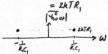
For noise of  $R_S$ , we should look into the noise at  $|\omega| = \omega_0 - \frac{1}{R_1 C_1}$ .
