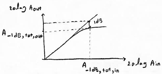
$$\Rightarrow 20 \log \left( \frac{A_{-1dB,\text{tot,out}}}{\alpha_1 \beta_1 A_{-1dB,\text{tot,in}}} \right) = -1 \text{ dB} \quad [2]$$
