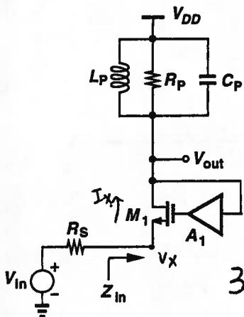
$$A) g_m (\Delta_1 V_{out} - V_x) = -V_{out} \left( \frac{1}{sL_p} + \frac{1}{R_p} + sC_p \right)$$
