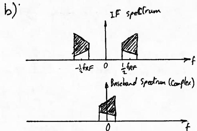
So this architecture will not work well with asymmetrically-modulated inputs in the presence of first LO third harmonic. This is because the third harmonic folds the signal on itself corrupting the information.
