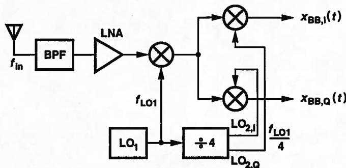
$$a) f_{in} - f_{LO_1} - \frac{f_{LO_1}}{4} = 0 \quad \therefore f_{in} = \frac{5}{4} f_{LO_1}$$
