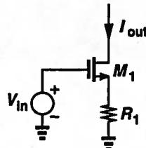
$$(a) \frac{1}{2}k(V_{in} - I_{out}R_1 - V_{th})^2 = I_{out}$$
