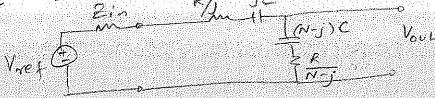
Due to the additional  $Z_{in}$  in the charging path, the settling should be increased.
