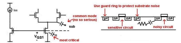
Different arguments for connecting substrate to analog ground and digital ground. Not clear. But the best way is to have a low-inductance connection to substrate.
