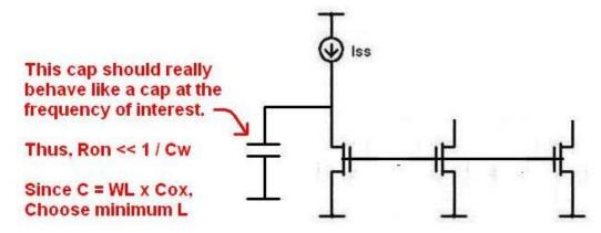
But must make sure on-resistance is sufficiently small (Q is high.)
