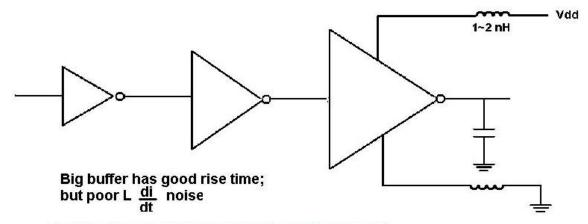
Need to simulate with bond wire inductance to Vdd
