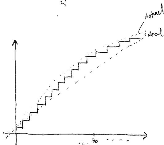
4. Consider a 6-bit flash ADC with 2x interpolation. The output of interest is the thermometer code generated by the latches.
