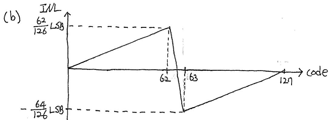
2. The 7-bit segmented current-steering DAC shown below employs 128 current sources nominally equal to  $I_0$ . Code 0 routes all of the tail currents to  $I_{out1}$  and code 127 routes all of the tail currents to  $I_{out2}$ . The output of interest is  $I_{out1} - I_{out2}$ . Neglect all mismatches.
