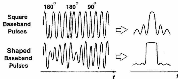
Thus, shaped QPSK has a variable amplitude (envelope) and hence requires a linear PA. GSMK, on the other hand, has a constant envelope and can operate with nonlinear PAs.
