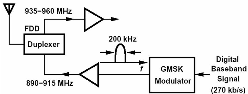
Now we have GPRS and EDGE. EDGE uses variable-envelope modulation and requires a linear PA.
