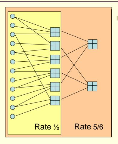
The higher-rate code is decoded by turning on the extra check-nodes and connecting them to the circuit
