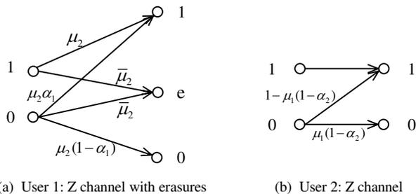
Fig. 11. Perceived channel by each decoder.
