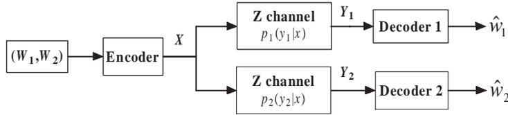
Fig. 7. Communication system for 2-user broadcast  $Z$  channels.
