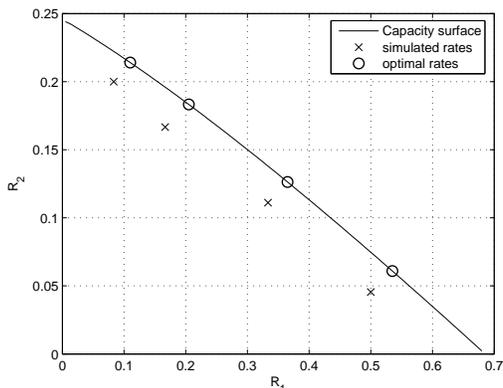
Fig. 12. Broadcast Z channel with crossover probabilities  $\alpha_1 = 0.15$  and  $\alpha_2 = 0.6$  for receiver 1 and 2 respectively: achievable capacity region, simulated rate pairs  $(R_1, R_2)$  and their corresponding optimal rates.
