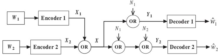
Fig. 8. Optimal transmission strategy for broadcast Z channels.
