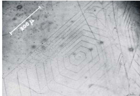
Figure 2.2: Frank-Read source in Si. Courtesy of Dash
