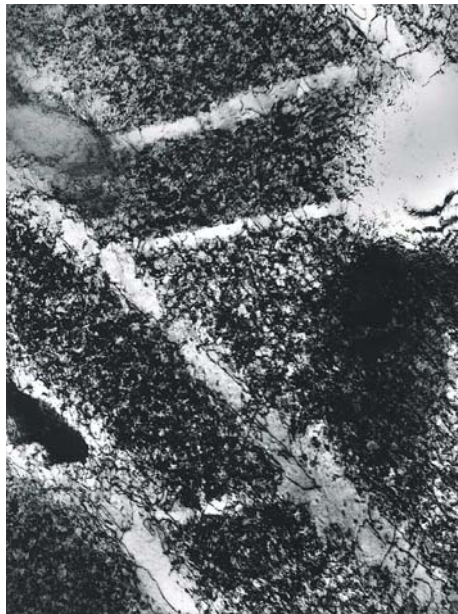
Figure 2.18: Dislocation channels in irradiated Cu. Courtesy of Singh.
