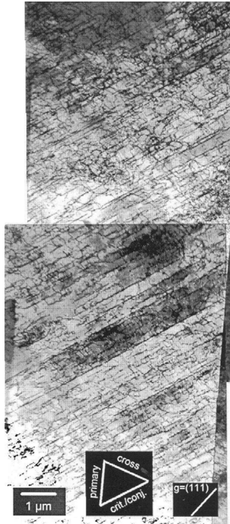
Figure 2.9: A fairly uniform structure of planar dislocation arrays are seen after completion of cyclic softening. No dipole arrays were found at this stage. The picture shows Cu-30%Zn cycled to \varepsilon = 3.4 \times 10^{-3} . The polycrystal is found to contain a fairly uniform structure of planar dislocation arrays
