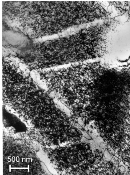
Figure 9.59: TEM picture of localized plastic flow emanating from internal inclusions in CuCrZr alloy, neutron-irradiated at 320 K to a dose level of 0.3 dpa and fatigue-tested at 320 K with a loading frequency of 0.5 Hz (Singh, Stubbins and Toft 2000a)
