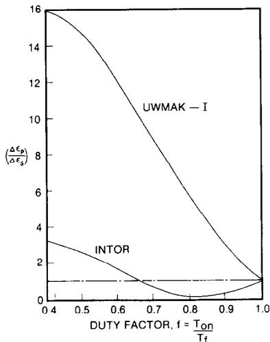
Fig. 2. The enhancement factor for UWMAK-I and INTOR as a function of the duty factor. Stainless steel at  $T=300^\circ\text{C}$ ,  $P=10^{-6}$  dpa/s,  $\rho_d=10^{12}/\text{m}^2$  for UWMAK-I and  $\rho_d=10^{14}/\text{m}^2$  for INTOR. All other material parameters are taken from ref [1].
