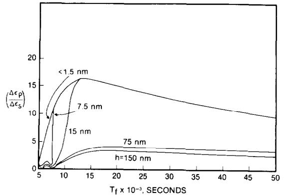
Fig. 1. The enhancement factor for nickel at 200°C as a function of the total cycle time for a given barrier height  $h$ .  $T = 5000\text{s}$ ,  $\rho_d = 2 \times 10^{13} \text{ m}^{-2}$ ,  $P = 10^{-6} \text{ dpa/s}$ , and all other material parameters are taken from ref. [1].
