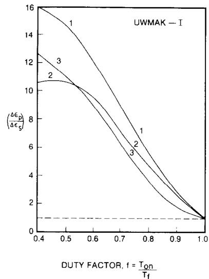
Fig. 3. The enhancement factor for UWMAK-I as a function of the duty factor, using different damage rates. Curve 1: dose-equivalent averaged damage rate; curve 2: equal instantaneous damage rates, dose not conserved; curve 3: equal instantaneous damage rates, dose conserved; All other conditions are the same as in Fig. 2.
