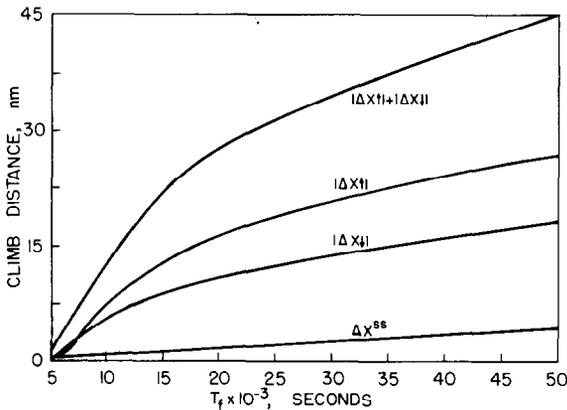
Fig. 3. Climb distances for pulsed and steady irradiation for nickel with  $T_{\text{on}} = 5000$  s as a function of the total cycle time.  $\rho_d = 2 \times 10^{13}/\text{m}^2$ ,  $T = 200^\circ\text{C}$ ,  $P = 10^{-6}$  dpa/s, and all other material parameters are taken from ref. [6].
