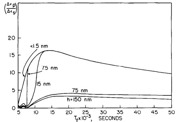
Fig. 4. The ratio of pulsed to steady irradiation creep strain for nickel at  $200^\circ\text{C}$  as a function of the total cycle time for a given barrier height  $h$ . Conditions are the same as in fig. 3.
