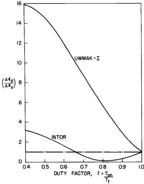
Fig. 6. The ratio of pulsed to steady irradiation creep strain for UWMMAK-I and INTOR as a function of the duty factor. Conditions are the same as in fig. 5.
