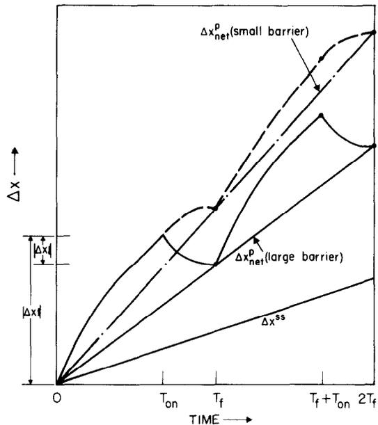
Fig. 2. Schematic illustrating climb distances during the on-time ( $|\Delta X \uparrow|$ ), during the off-time ( $|\Delta X \downarrow|$ ), for steady irradiation ( $\Delta X_{ss}$ ), and net climb distances for small and large barriers ( $\Delta X_{net}^p$ ).
