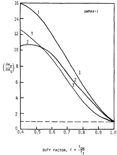
Fig. 7. The ratio of pulsed to steady irradiation creep strain for UWMAK-I as a function of the duty factor, using different damage rates. Curve 1: dose-equivalent averaged damage rate; curve 2: equal instantaneous damage rates, dose not conserved; curve 3: equal instantaneous damage rates, dose conserved.
