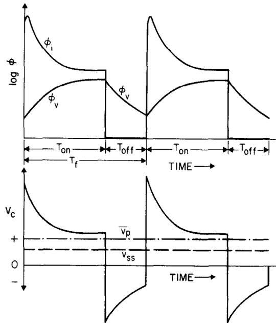
Fig. 1. Schematic of point-defect fluxes  $\phi_{i,v} = (ZDC)_{i,v}$  and dislocation velocities.  $\bar{v}_p$  and  $\bar{v}_{ss}$  are the average dislocation velocities during pulsed and steady irradiation, respectively.
