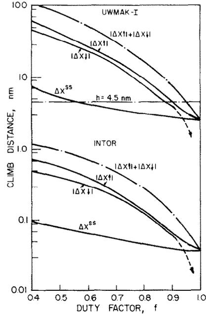
Fig. 5. Climb distances for pulsed and steady irradiation for the UWMAK-I and INTOR reactor designs as a function of the duty factor. The first wall was assumed to be stainless steel operating at  $T=300^\circ\text{C}$ ,  $P=10^{-6}$  dpa/s,  $\rho_d=10^{12}/\text{m}^2$  for UWMAK-I and  $\rho_d=10^{14}/\text{m}^2$  for INTOR. All other material parameters are taken from ref. [6].
