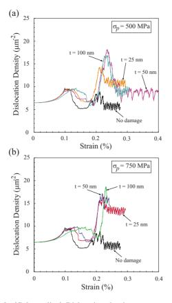
FIG. 2. (Color online) Dislocation density versus strain for a  $D=0.75 \ \mu \text{m}$  micropillar having two precipitate strengths: (a)  $\sigma_p=500$  MPa and (b)  $\sigma_p=750$  MPa. Both cases produce an initial increase in dislocation density, however this density persists into the steady-state regime for the larger precipitate strength.
