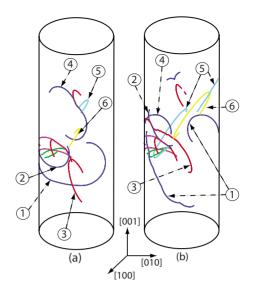
FIG. 1. (Color online) Microstructure of a  $D=0.75 \ \mu \text{m}$  micropillar at 0.17% strain. (a) No damage layer. (b) Damage layer depth t=100 nm and precipitate strength of  $\sigma_p=750 \text{ MPa}$  is used. The precipitates are not plotted for clarity. The numbers encircled reference the same dislocations in both simulations.
