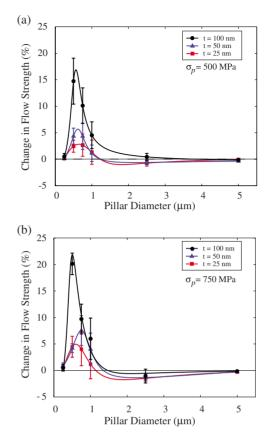
FIG. 3. (Color online) The average percentage change in the computed flow strength, for different micropillar sizes and precipitate layer depth. (a)  $\sigma_p = 500$  MPa; (b)  $\sigma_p = 750$  MPa. The error bars are the standard deviation of the simulated results from the average and the solid lines represent the best fit for each damage depth.
