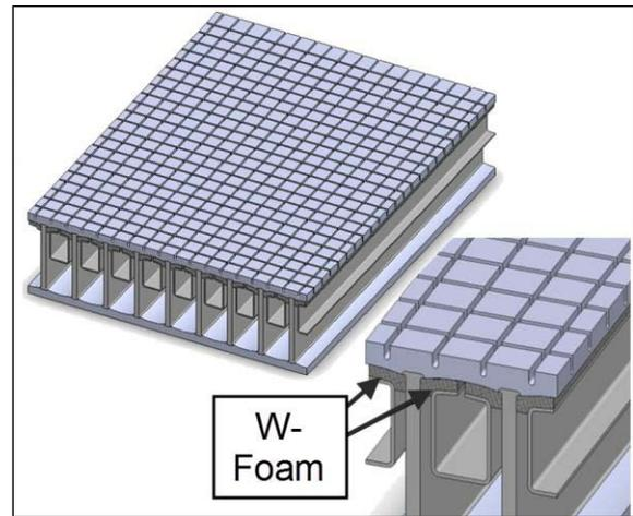
Fig. 4. CAD model of an early flat-plate divertor concept using foam to enhance heat transfer.
