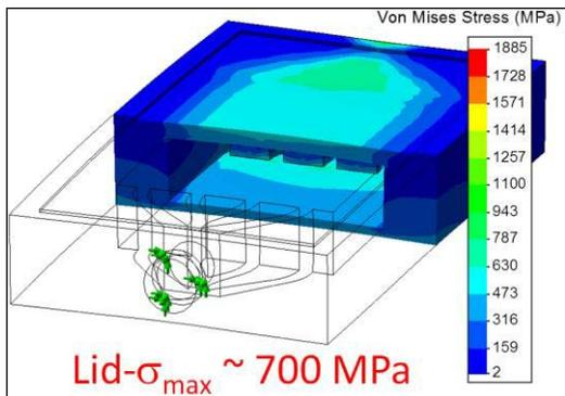
Fig. 9. FEA Von Mises Stress results for flat-plate HX prototype design [note: print copy is b&w, but color online].
