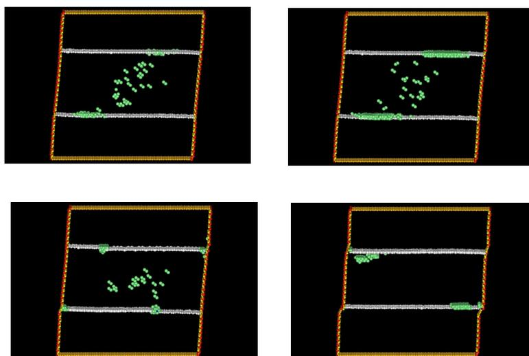
Figure 7: MD simulations of a twinned copper nano-crystal showing the process of twin boundary motion resulting from homogeneous dislocation loop nucleation
