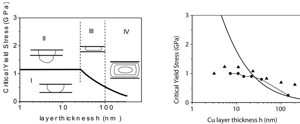
Figure 4: (a) Left, Deformation regimes for layered nano-composites determined by DD simulations (b) Right, Yield strength of a Ni-Cu layered thin film as a function of the layer thickness. Solid line: Freund's formula, triangles: experimental results [Misra, et al.[7]], and circles: current simulation results [11]
