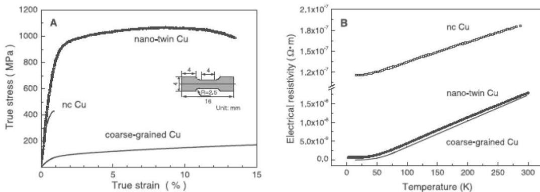
Figure 2: (a) Left, Typical tensile stress-strain curve of nano-twin Cu, nano-grain Cu of grain size of 30 nm, and coarse-grained Cu; (b) right, measured temperature dependence of electrical resistance of nano-twin Cu, nano-grained Cu, and coarse-grained Cu. [1]
