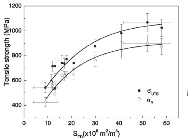
Figure 9: Experimental measurements for the dependence of the strength on the twin boundary area [1]
