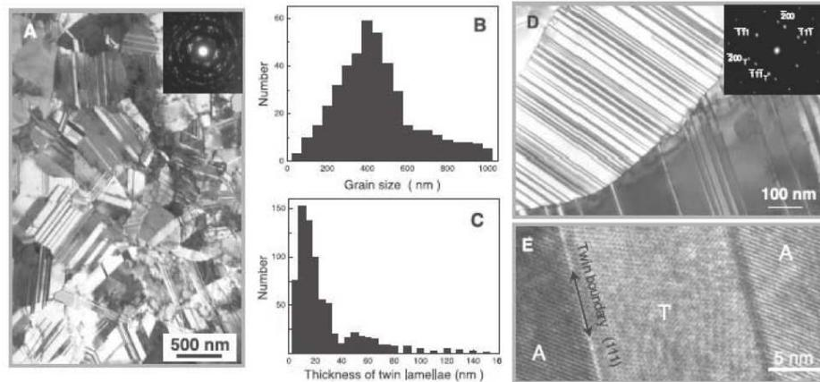
Figure 1: 1(A) A bright-field image of an as-deposited Cu. (B) Statistical distribution of grain size, (C) Statistical distribution of thickness of twin lamellae. (D) Nano twins are parallel to 111 planes. (E) High resolution of twin sequence of ATATA [1]
