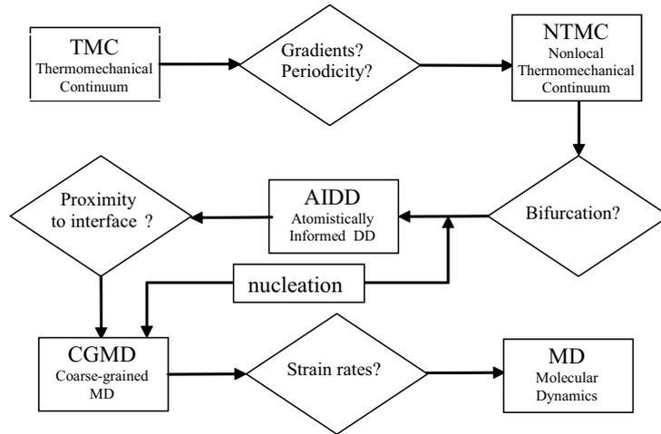
Figure 8: Model error estimators and adaptive model selection
