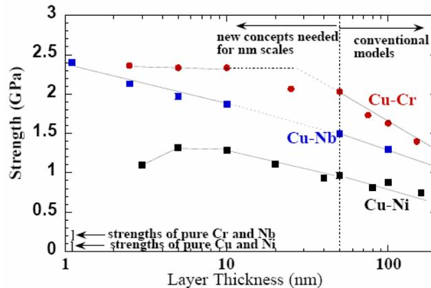
Figure 3: Dependence of Nano-layer composite strength on the layer thickness. Experimental data of Misra et al., LANL [5, 6, 7]
