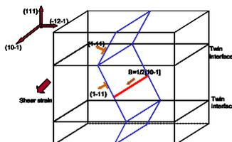
Figure 5: Schematic illustration of the simulation conditions for twinned copper nano0crystals (Lan Li, UCLA, unpublished results)
