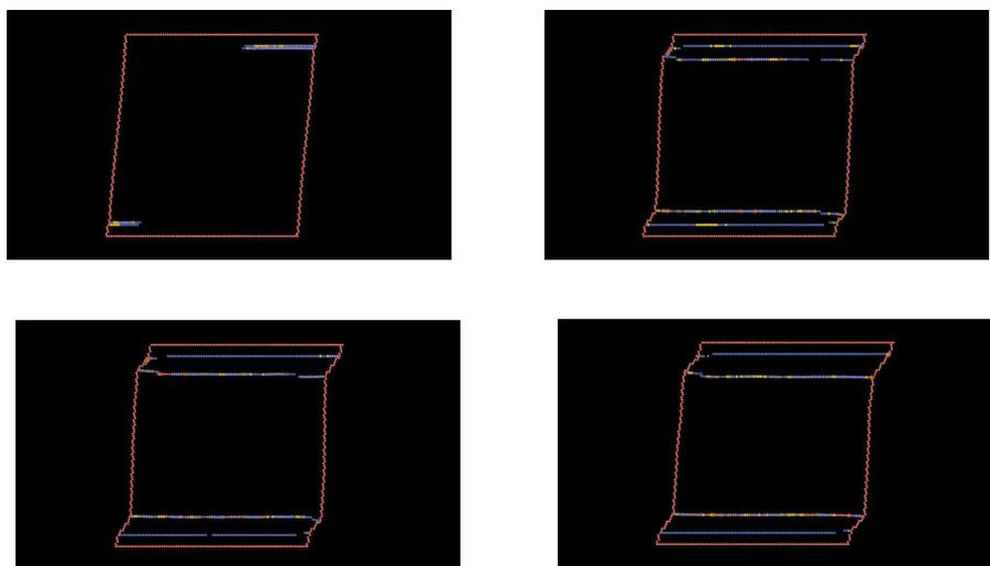
Figure 6: Results of MD simulations for a sequence of snap-shots showing the development of twins in a perfect copper crystal under shear deformation (Lan Li, UCLA, unpublished results)
