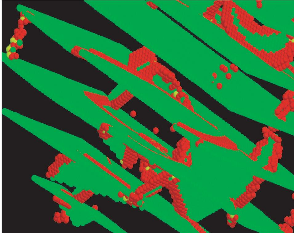
Figure 5.29: Dominant deformation modes of nano-twinning copper crystals. The figure shows the operation of the Twin Boundary Migration (TBM) mechanism (see fourth boundary from the bottom), and Mechanical Twinning (MT) as is clear in the double layers bound by Shockley partial dislocations.
