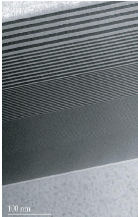
Figure 1.1: A multi-period ZrC/Si Nano-Laminate[85].
