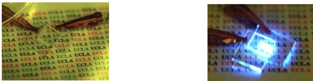
A transparent blue-emission polymer SLED. Left, the picture of an unbiased SLED, it shows the transparent devices. Right, the picture of a biased SLED, it shows strong blue electrochemiluminescence.
