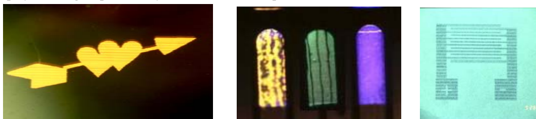
Pictures of polymer devices fabricated via hybrid ink-jet printing technology. Left, the picture of a polymer light-emitting logo. Middle, the picture of multi-color organic light-emitting diodes. Right, inter-digitated electrodes fabricated from conducting polymer.
