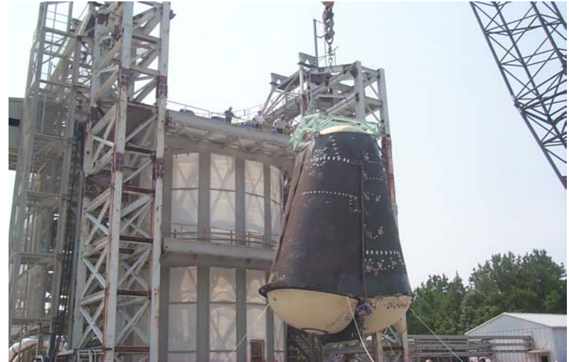
X-33 LH2 composite tank failure
