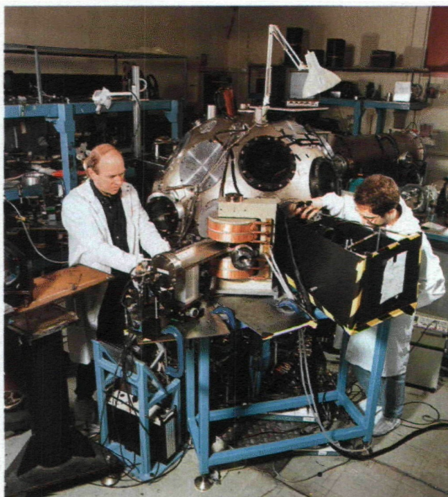
Preparing a short-pulse electron acceleration experiment using the VULCAN laser at the Rutherford Appleton Laboratory.
