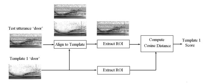
Figure 2: Block diagram of the similarity score extraction using the example word 'door' from template child 1.
