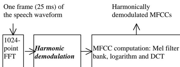
**Figure 6:** Block diagram of the harmonically demodulated MFCCs.
