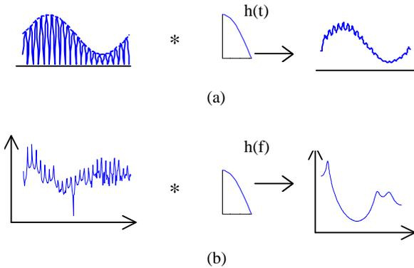
**Figure 3:** (a) Envelope detector for AM demodulation. First, full wave rectification is applied, and then the signal is convolved with the impulse response of a low-pass filter. The x-axis here is time. (b) Similar process to (a), except that it is done in the frequency domain by using the magnitude of a speech spectrum. The x-axis here is frequency.
