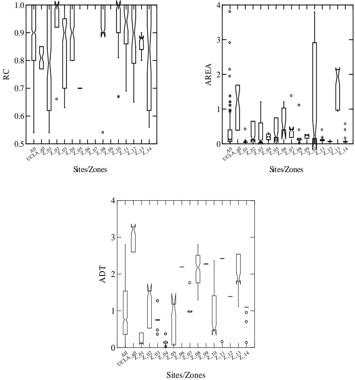
**Fig. 3.4B.** Site-specific Characteristics for Combined UCLA Sites (UCLA\_all), Combined Other Sites (All), and 14 Caltrans Zones (e.g. Z\_01 is Zone 1) ; Runoff Coefficient (RC, Dimensionless), Catchment Area (AREA, ha), and Average Daily Traffic (ADT,  $\times 10^5$  vehicles/day).
