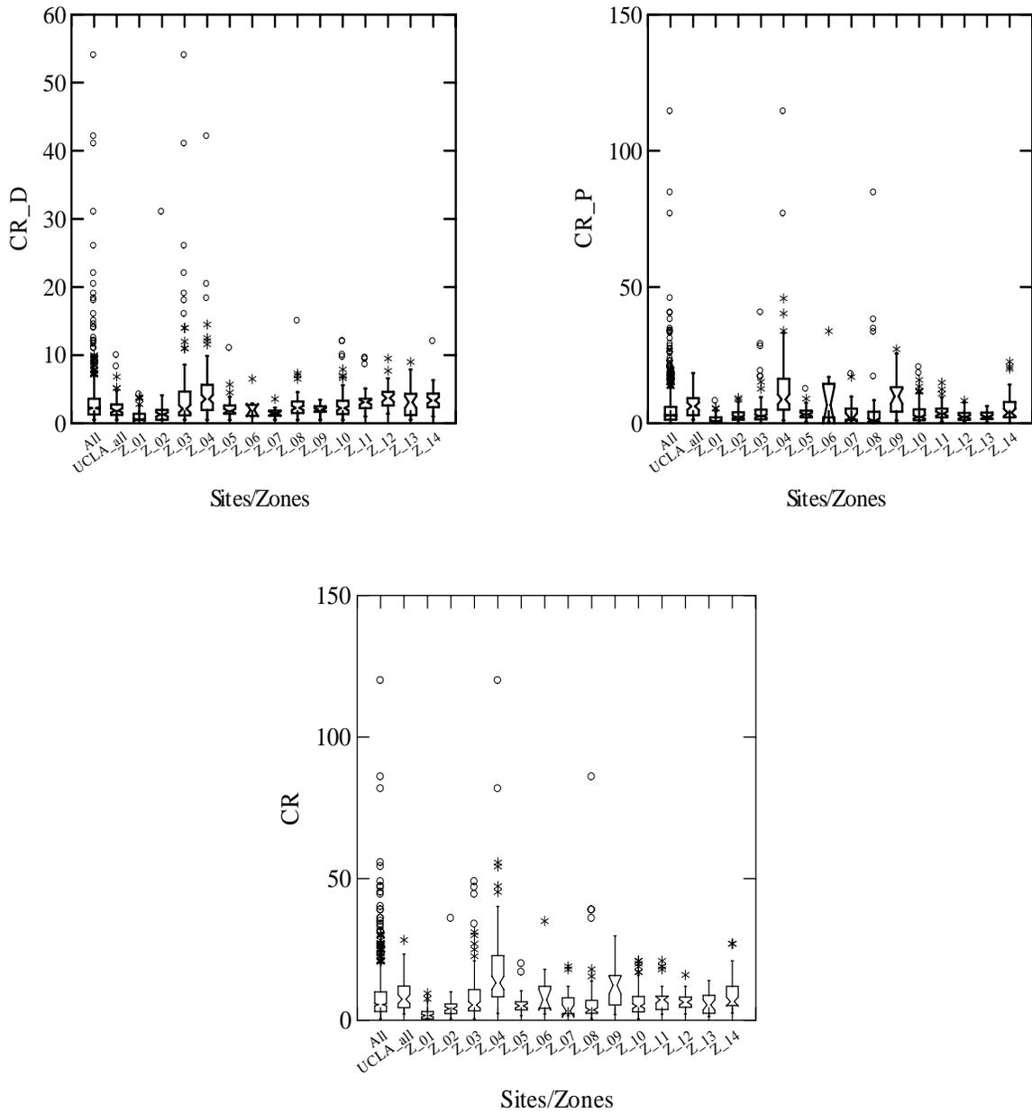
**Fig. 3.5B.** EMC ( $\mu\text{g/L}$ ) Characteristics for Combined UCLA Sites (UCLA\_all), Combined Other Sites (All), and 14 Caltrans Zones (e.g. Z\_01 is Zone 1) for Dissolved (CR\_D), Particulate (CR\_P), and Total (CR) Chromium
