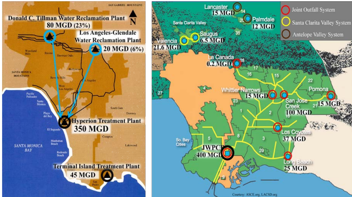
Figure 1.1 Treatment plant system operated by LA City Bureau of Sanitation (left) and LA County Sanitation District (right) (American Society of Civil Engineers, 2012; LA County Sanitation District, 2012).
