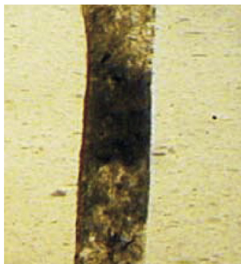
Fig. 5 – Silicon membrane section seen under reflective (left image) and polarised (right image) light. Polymeric substances (silicone) are not optically active, while crystalline formations (mica scales) interact with the polarised light and rotate the plane of polarisation (bright band in the right image).
