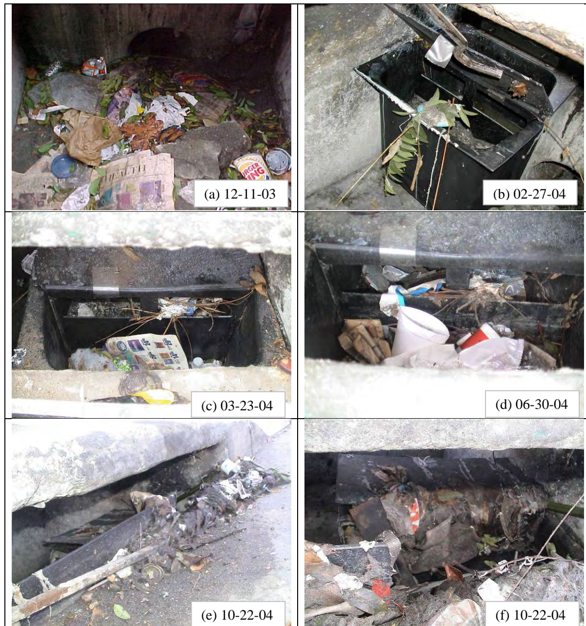
Figure 4-16. Field inspection photos showing the condition of Hydro-Kleen at the intersection of Washington and Walton.
