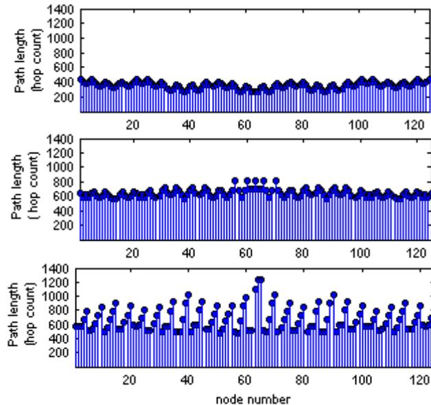
Figure 9. Average path length, in terms of hop count, for the grid network, in case of: SPR, SMR, CSR (from top to bottom)
