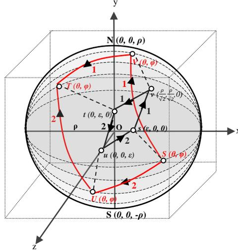
Figure 5 (a). Two Euclidian paths (1, 2) in the grid are shown in black and two Spherical paths (1, 2) on the surface of the sphere are shown in red.
