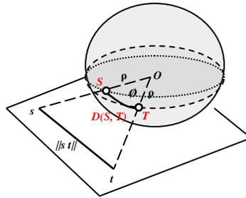
Figure 5 (b). Grid to spherical Projection diagram (Lemma 1)
