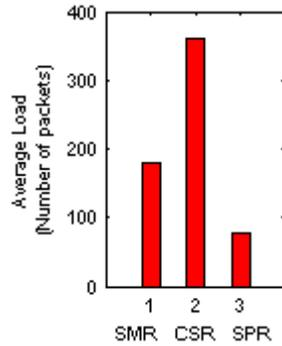
Figure 7 (b). Average load in the boundary of the grid network for: (1) SMR (2) CSR (3) SPR
