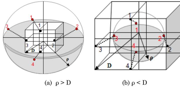
Figure 2. The mapping of points from 3D grid to projected points on the surface of various spheres of different sizes:
