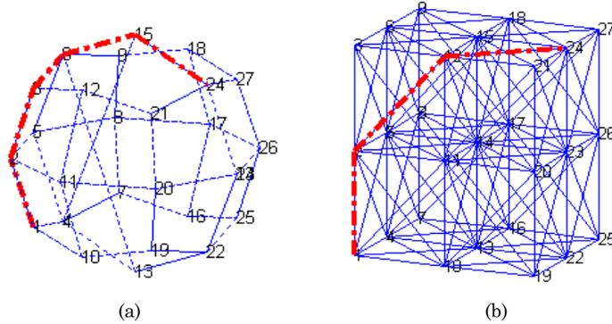
Figure 4. Blue lines show the network topology and connectivity for a 3D sphere and a 3x3x3 grid. Red line showing the routing path from source node to the destination node: (a) Spherical Mapping based Routing (SMR) (b) Reverse Spherical Mapping based Routing
