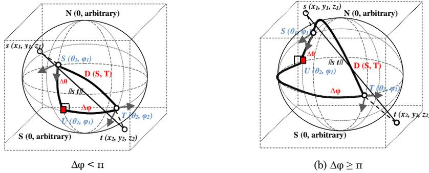
Figure 3. The spherical distance calculation between points  $S$  and  $T$  on the surface of the sphere.
