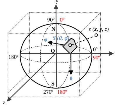
Figure 1. Spherical coordinates based mapping from a cube to a sphere: one to one mapping from a node  $s$  in cube to a node  $S$  on sphere
