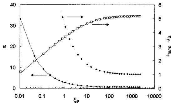
FIG. 2. Decrease of floating potential  $\eta_f$  ( $\square$ ) with decreasing  $\xi_p=R_p/\lambda_D$  due to the increase in sheath area as measured by  $\alpha$  ( $\bullet$ ) and  $\alpha/\alpha_0$  ( $\blacklozenge$ ). The line through the  $\eta_f$  points is an analytic fit.
