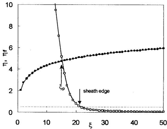
FIG. 1. The radial potential profile  $\eta(\xi)$  ( $\square$ ) and the floating potential condition  $\eta_f(\xi)$  ( $\bullet$ ) for the case  $J=10$ ,  $\xi_p=15$  in argon. The dashed line indicates the “sheath edge” where  $\eta=\frac{1}{2}$ , but for cylinders the plasma is not quasineutral there.
