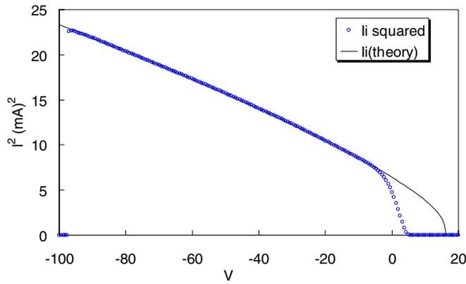
**Figure 10.** An ABR fit to the same data as in figure 8. The result is  $n = 1.06 \times 10^{12} \text{ cm}^{-3}$  and  $KT_e = 2.3 \text{ eV}$  ( $\xi_p = 5.8$ ).
