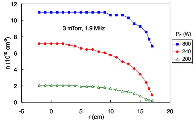
**Figure 2.** Density profiles in the ICP of figure 1. The density is peaked on axis even though the skin depth of the RF is only 3 cm.
