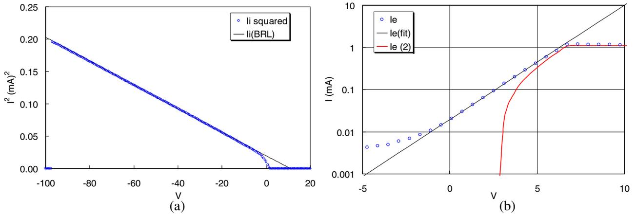
**Figure 6.** Same data as in figure 5 but analyzed with the BRL theory. The result is  $n = 0.81 \times 10^{11} \text{ cm}^{-3}$  and  $KT_e = 1.60 \text{ eV}$  ( $\xi_p = 1.93$ ).
