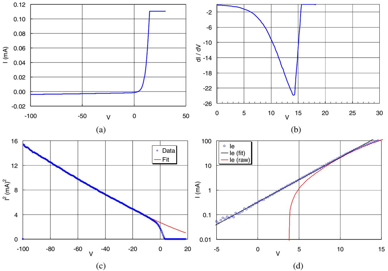
**Figure 4.** (a) Entire  $I$ - $V$  curve; (b) derivative of  $I$ - $V$  curve with a sharp minimum indicating the plasma potential; (c) plot of  $I_i^2$  versus  $V_p$  (points) and straight-line fit (—); (d) semilog plot of  $I_e$  versus  $V_p$  and straight-line fit to a Maxwellian.
