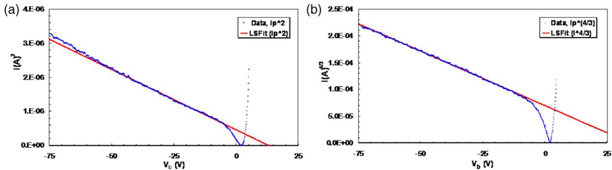
Figure 22. Ion curves (a)  $I^2-V$  and (b)  $I^{4/3}-V$ , showing a better fit with  $I^{4/3}$ .
