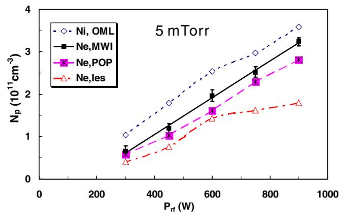
**Figure 14.** The data of figure 13 compared with  $n_e$  from POP and electron saturation current  $I_{es}$ .
