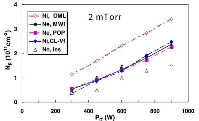
**Figure 18.** Power scan of density at 2 mTorr with various diagnostics.
