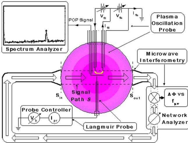
**Figure 3.** Conceptual cutaway (top) view of experimental setup, including the essential elements of the diagnostics. Also shown (dotted lines) is the plasma volume subtended by the MWI signal beam path, which encompasses the region sampled by the POP and Langmuir probes.
