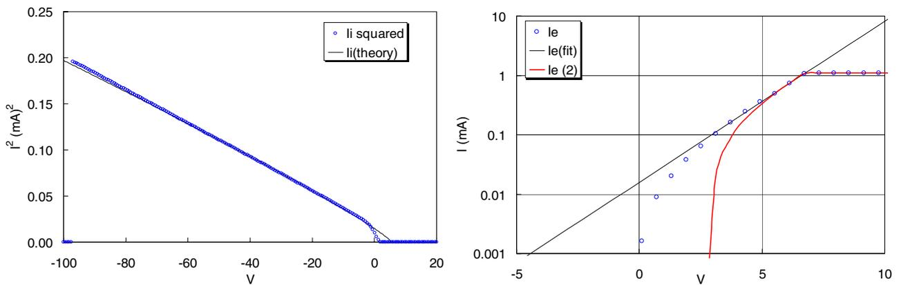
**Figure 7.** Same data as in figure 4 but analyzed with the ABR theory. The result is  $n = 0.23 \times 10^{11} \text{ cm}^{-3}$  and  $KT_e = 1.60 \text{ eV}$  ( $\xi_p = 1.03$ ).
