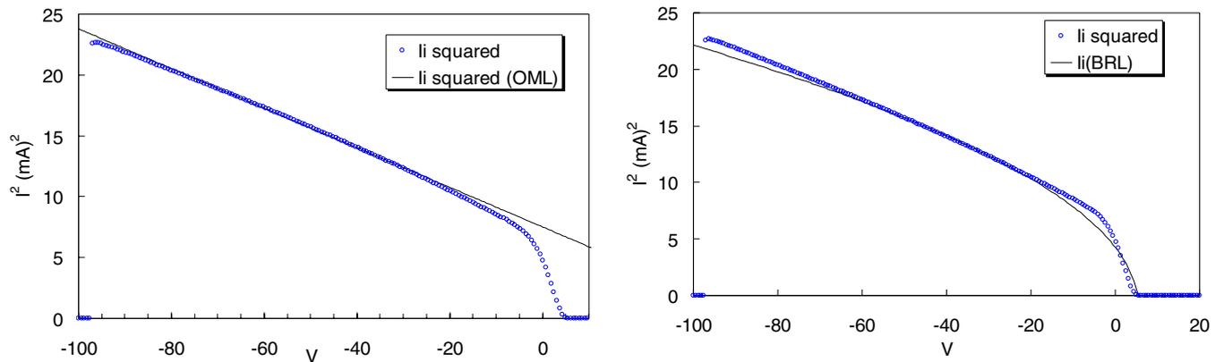
**Figure 8.** An OML fit to the ion current in a high-density plasma. The result is  $n = 1.3 \times 10^{12} \text{ cm}^{-3}$  and  $KT_e = 3.0 \text{ eV}$  ( $\xi_p = 5.6$ ).
