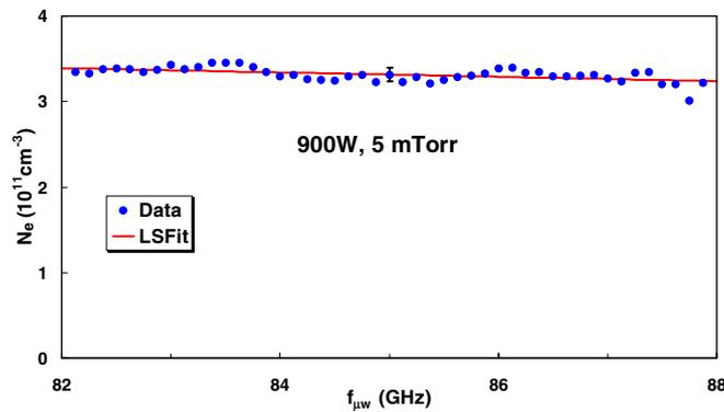
**Figure 11.** Plasma density measured by MWI at various frequencies, showing absence of spurious effects.
