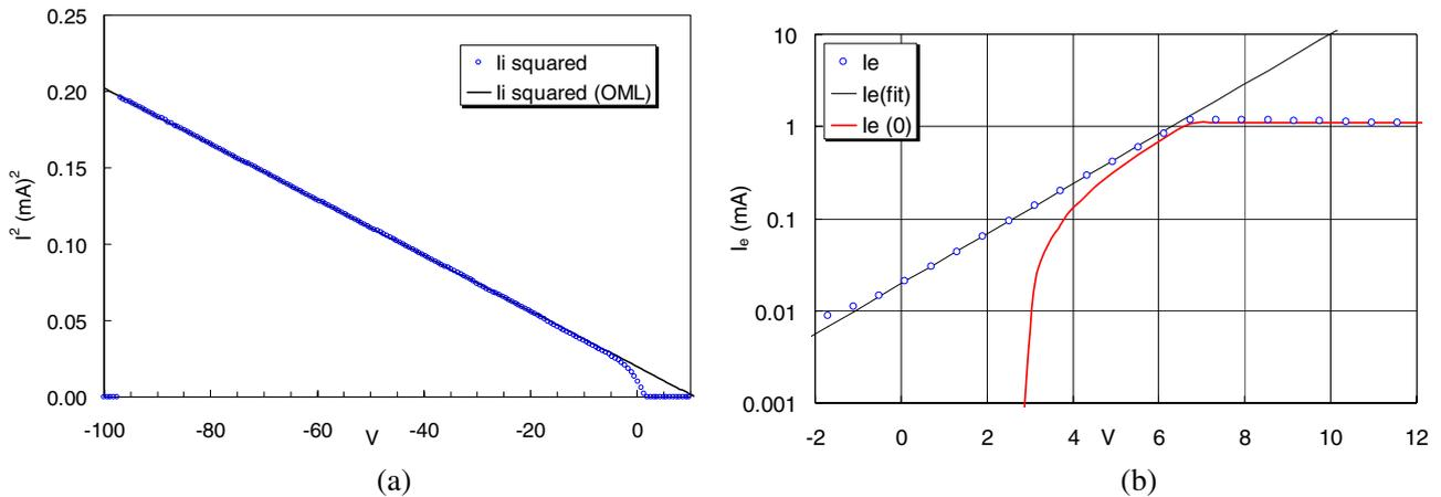
**Figure 5.** (a) Plot of  $I_i^2$  versus  $V_p$  as in figure 4(c). (b) Semilog plot of  $I_e$  versus  $V_p$  and a Maxwellian fit, as in figure 4(d). For convenience the  $I_e$  data were taken only up to 1 mA. The OML result is  $n = 0.80 \times 10^{11} \text{ cm}^{-3}$  and  $KT_e = 1.60 \text{ eV}$  ( $\xi_p = 1.92$ ).
