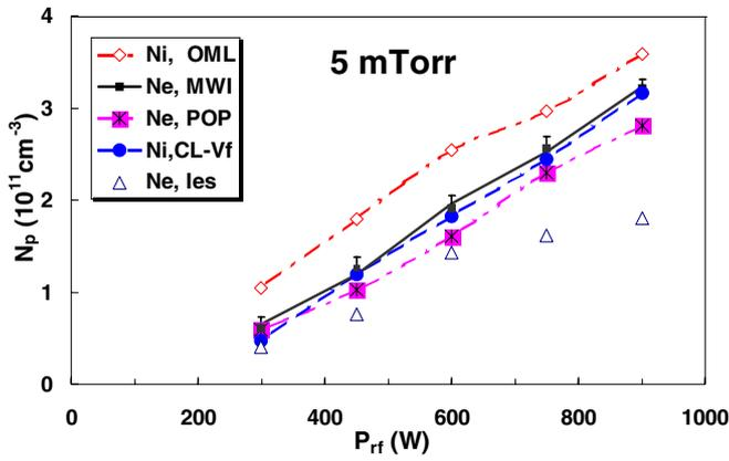
**Figure 19.** Power scan of density at 5 mTorr with various diagnostics.
