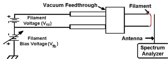
**Figure 12.** Diagram of POP apparatus.
