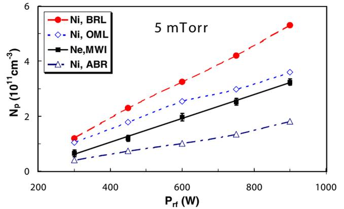
**Figure 13.** Plasma density measured with MWI (solid black line), compared with probe data analyzed with various theories.
