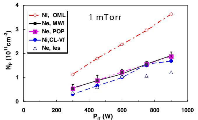
**Figure 17.** Power scan of density at 1 mTorr with various diagnostics, taken on axis ( $r = 0$ ).
