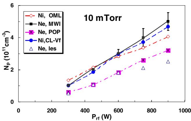
**Figure 20.** Power scan of density at 10 mTorr with various diagnostics.
