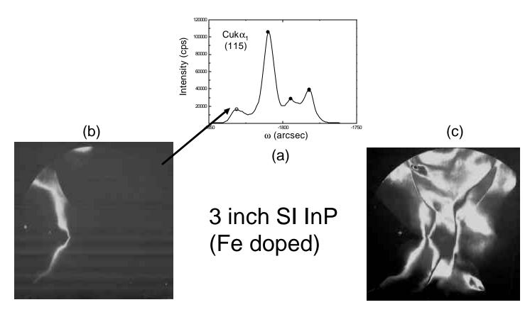
(a) is the rocking curve of the 3 inch InP substrate showing four peaks, (b) is the x-ray topograph taken at the left most peak of the rocking curve and (c) is the x-ray topograph which is a composite of topographs taken at the top of each of the four peaks. The x-ray topograph shows large tilt and mosaic regions indicating poor crystalline quality.
