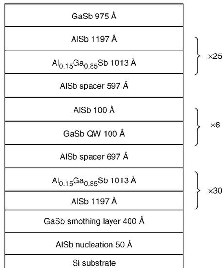
**Fig. 1** Monolithic VCSEL structure schematic shows GaSb/AlSb QWs in half-wave cavity spacer surrounded by AlGaSb/AlSb DBRs
