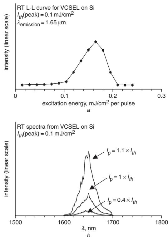
**Fig. 2** RT-PP lasing results at  $1.65 \mu\text{m}$  from VCSEL grown on Si
