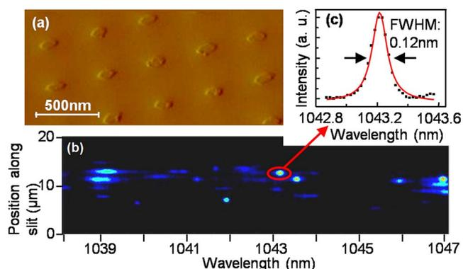
FIG. 1. (Color online) (a) AFM image of capped sample. (b) Typical spectrum recorded with 180 s integration time. The y axis corresponds to the spatial axis along the spectrometer slit while the x axis denotes wavelength. Each peak is from a single QD emission. The peaks are most likely from the ground state due to the low temperature and the excitation intensity. (c) Intensity profile of one QD state with a Lorentzian line shape.
