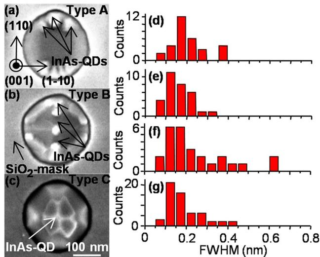
FIG. 2. (Color online) [(a)–(c)] Morphology of patterned QDs grown on the three different kinds of pyramids. The histograms show the distribution of the linewidth for a certain set of pyramids: (d) data from type A, (e) data from type B, and [(f)–(g)] data from type C. Each bin in a histogram covers a range of 0.05 nm. The data were taken at a temperature of 6 K.
