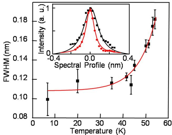
FIG. 3. (Color online) Temperature dependence of the FWHM of one QD. The linewidth increases suddenly at 40 K. Inset: intensity profiles at 6.8 K (FWHM=0.1 nm) and 45 K (FWHM=0.18 nm). Uncertainty in Lorentzian curve fitting represents the dominant contribution to the error bars shown.
