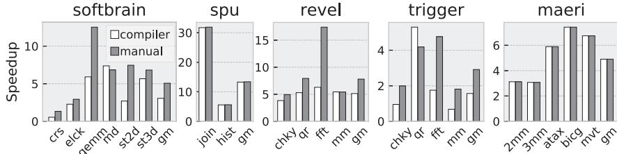
Fig. 4. Compiler versus manual-tuned performance.
