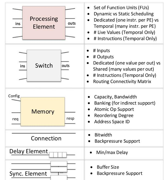
Fig. 3. Decoupled spatial architecture components.
