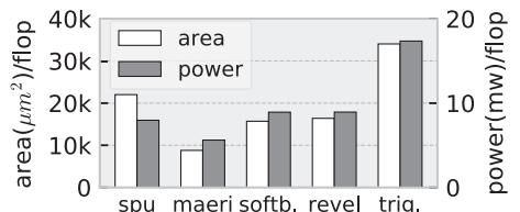
Fig. 5. Area and power normalized by peak FLOPs.
