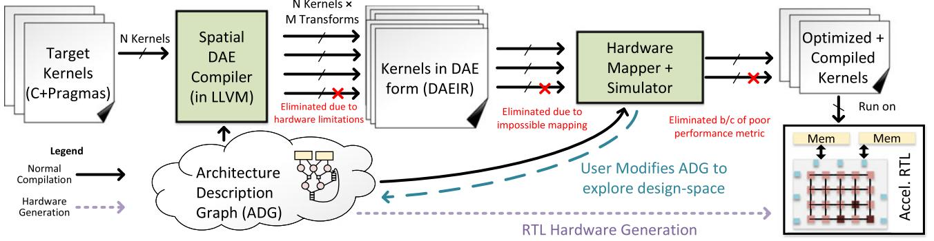
Fig. 2. Overview of DAEGEN architecture design framework.
