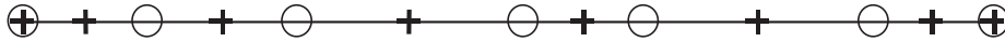
Fig. 5. O's are nodes and +'s are node-to-node midpoints. O's and +'s are the sampling points of the body forces in SC nodal (rect.) and SC nodal (trap.), respectively.
