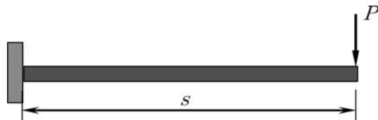
Fig. 9 Clamped-free straight beam subjected to a tip load
