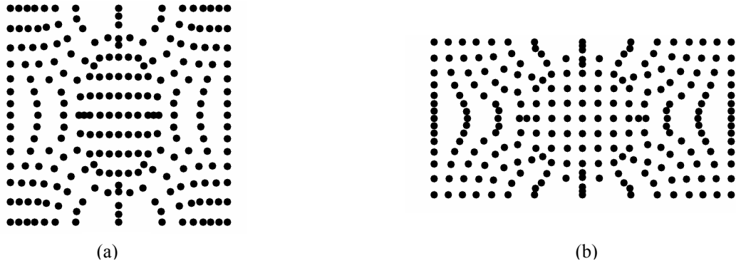
Figure 7 Displacement fields with 3% magnetostrictive eigen-strain for tension test: (a) Local fluctuating deformation; (b) Microscopic total deformation
