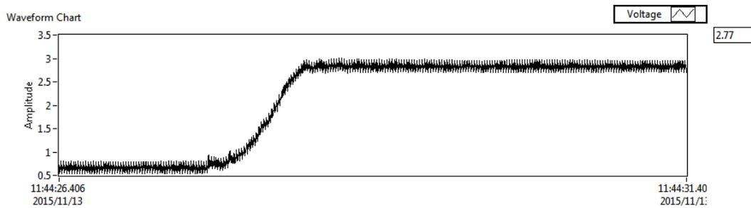
Figure 4.6: Load cell output with the amplifying circuit.
