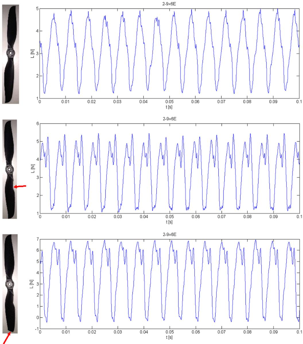
Figure 5.8: Vibration of unbalanced propellers.
