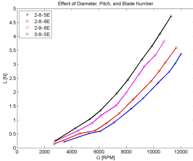
Figure 5.4: Effect of propeller diameter, pitch, and blade number on lift force.
