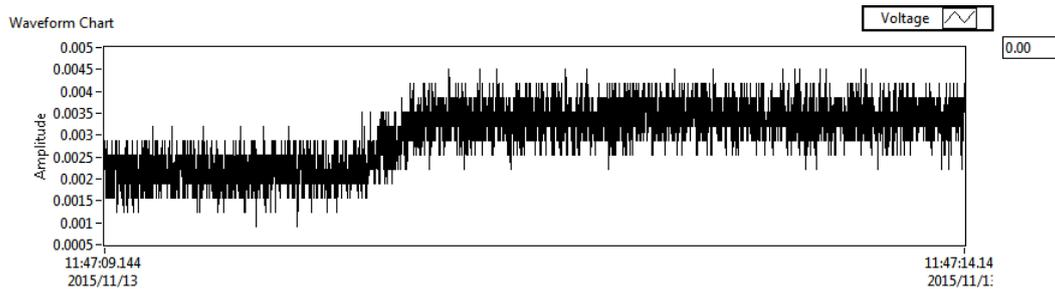
Figure 4.4: Load cell output without the amplifying circuit.
