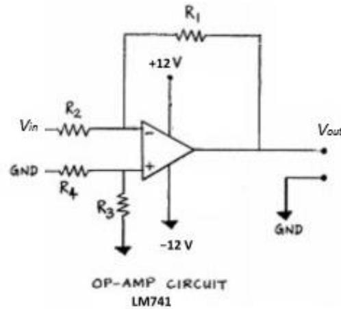
Figure 4.5: Designed amplifying circuit.<sup>[4]</sup>
