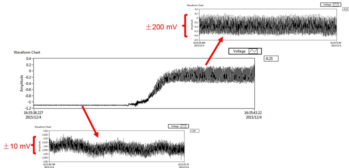
Figure 4.10: Transient step response.
