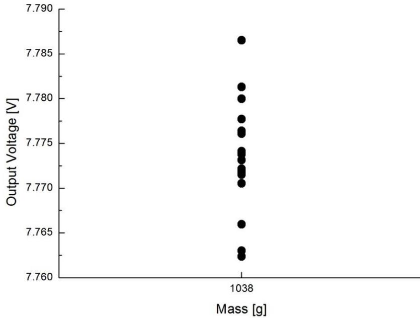
Figure 4.9: Output voltage for 1038-gram tension.
