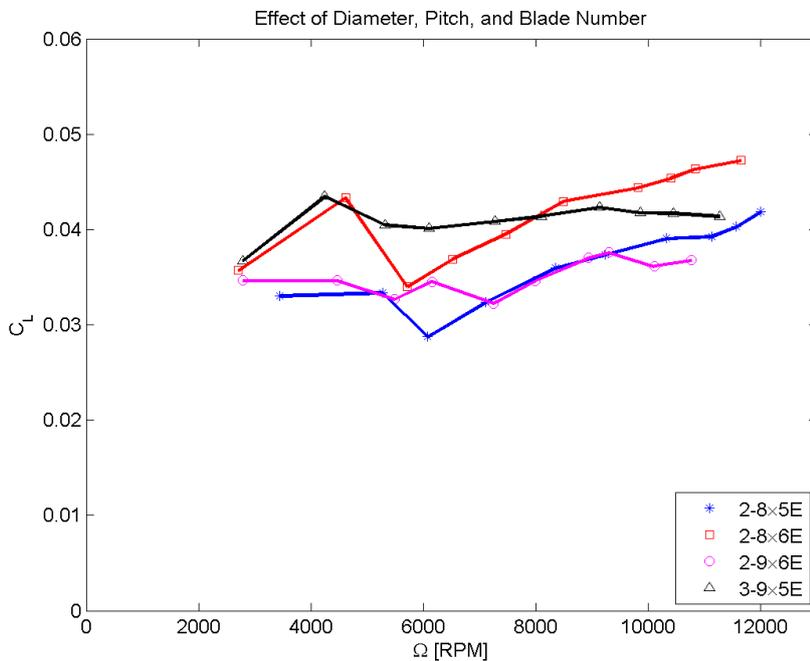
Figure 5.5: Effect of propeller diameter, pitch, and blade number on lift coefficient.
