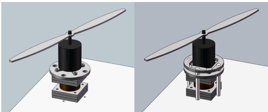
Figure 3.7: Motor fixture.
