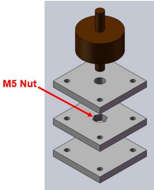
Figure 3.6: Load cell fixture.
