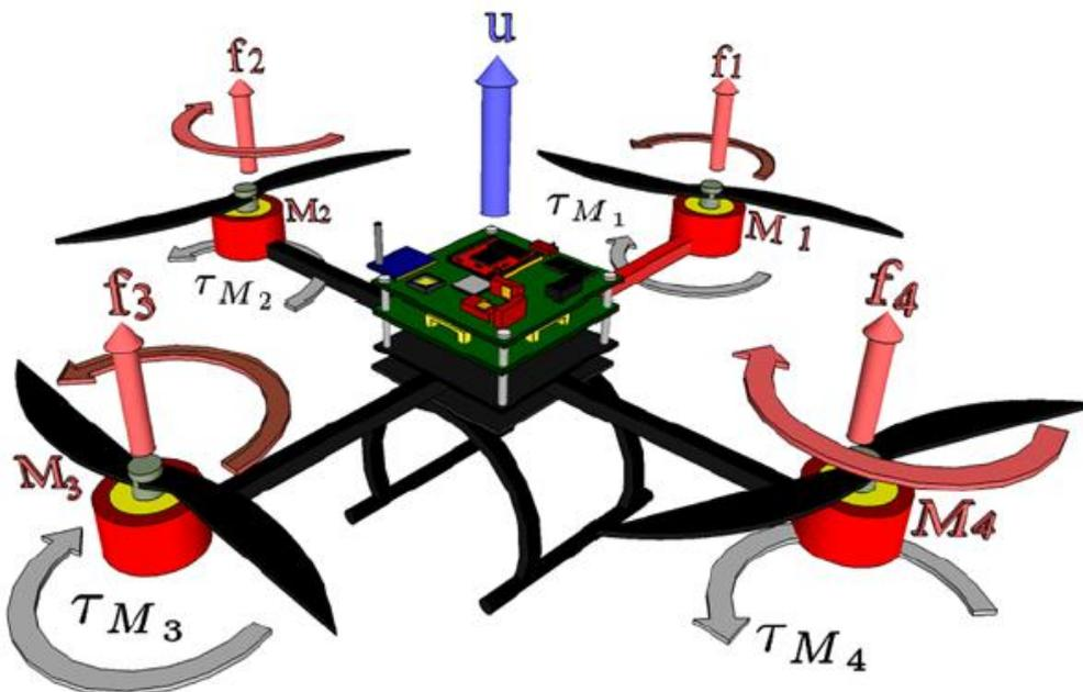
Figure 1.1: Free body diagram of the quadrotor. Retrieved from <http://www.mathworks.com/matlabcentral/answers/109279-modelling-a-quadrotor-with-simmechanics>.
