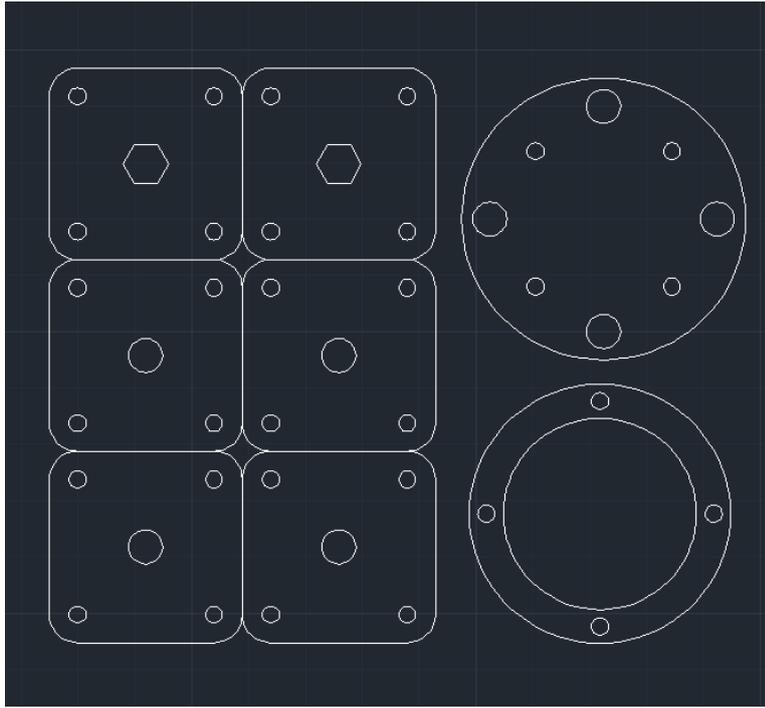
Figure F-2: AutoCAD of the load cell fixture.
