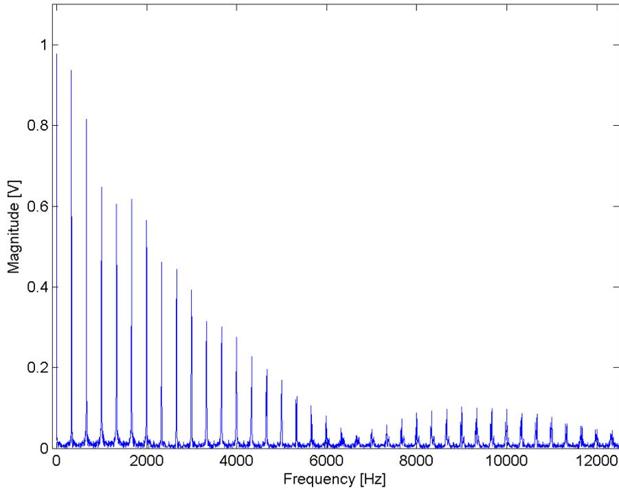
Figure 4.3: FFT of output signal.
