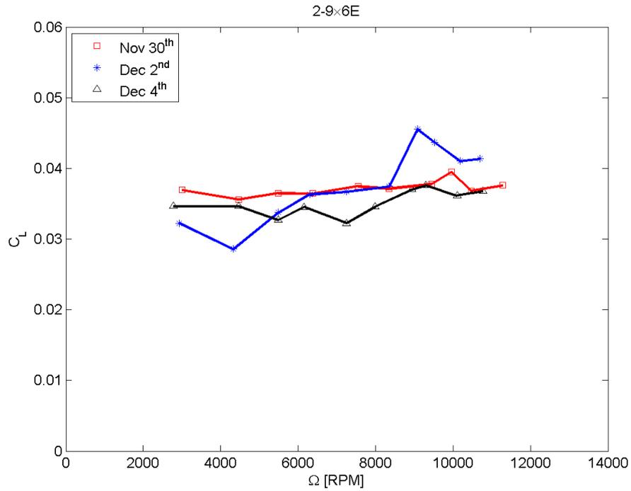
Figure 5.3: Lift coefficient vs. rotating speed.
