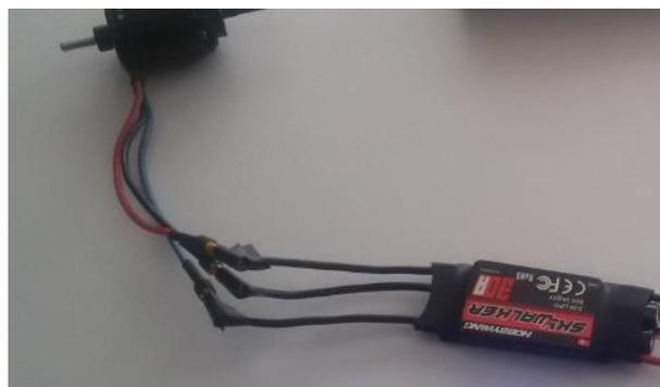
Figure 3.9: Connection between the motor and ESC.
