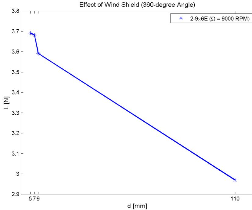
Figure 5.7: Effect of distance between the wind shield and the propeller on lift force.
