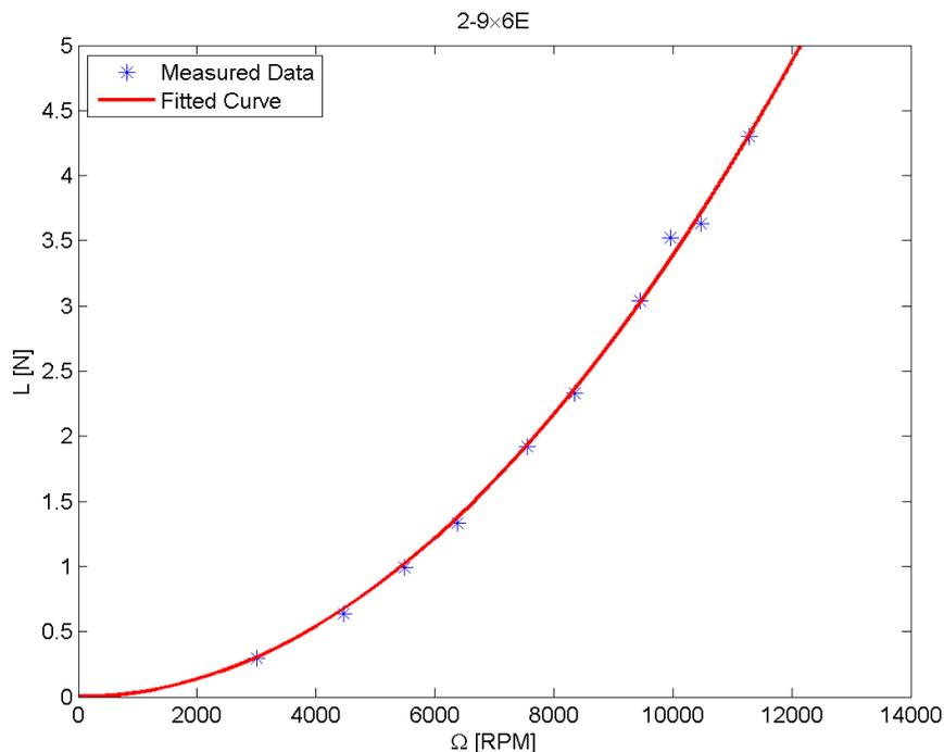
Figure 5.1: Lift force vs. rotating speed.
