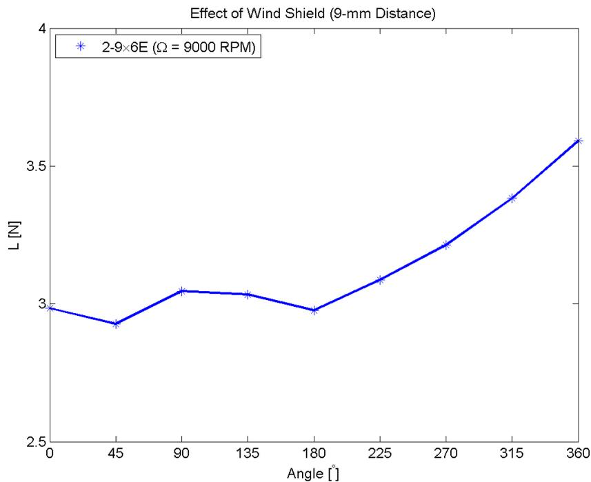
Figure 5.6: Effect of wind shield angle on lift force.
