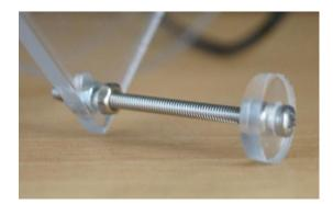
Figure 4.7: Auxiliary wheel on the power supply side.
