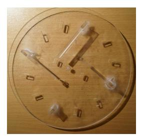
Figure 4.1: Vehicle wheel with pawls.
