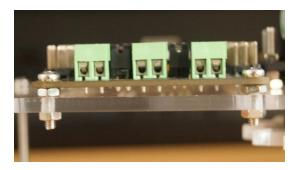
Figure 4.5: Fix of the control board.
