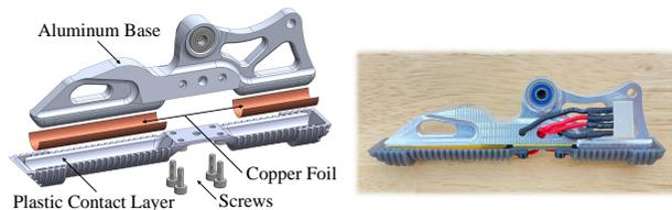
Fig. 4. BRUCE contact sensing foot. On the right is the hardware assembly and on the left is the exploded view of CAD model. For the assembly, the two copper foils are glued to the plastic contact layer, which is then attached to the aluminum base using screws.
