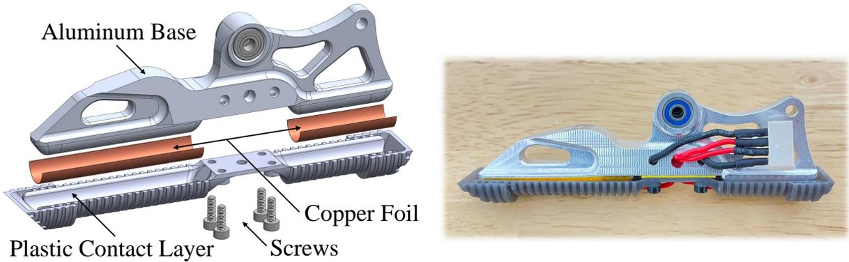
Figure 2.5: BRUCE contact sensing foot V1. On the left is the exploded view of the CAD model and on the right is the hardware assembly. For the assembly, the two copper foils are glued to the plastic contact layer, which is then attached to the aluminum base using screws.
